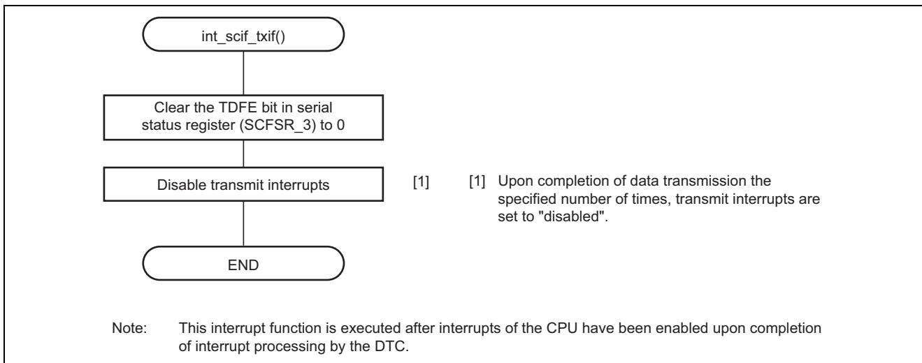
**Figure 14 Flow for Handling Transmit Interrupts in Asynchronous Mode**
