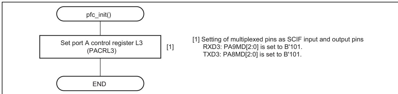
Figure 13 Flow for Setting Up the Pin Function Controller
