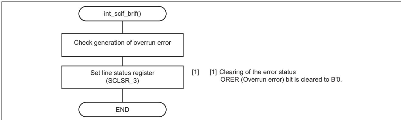
**Figure 16 Flow for Handling Receive Error Interrupts in Asynchronous Mode**
