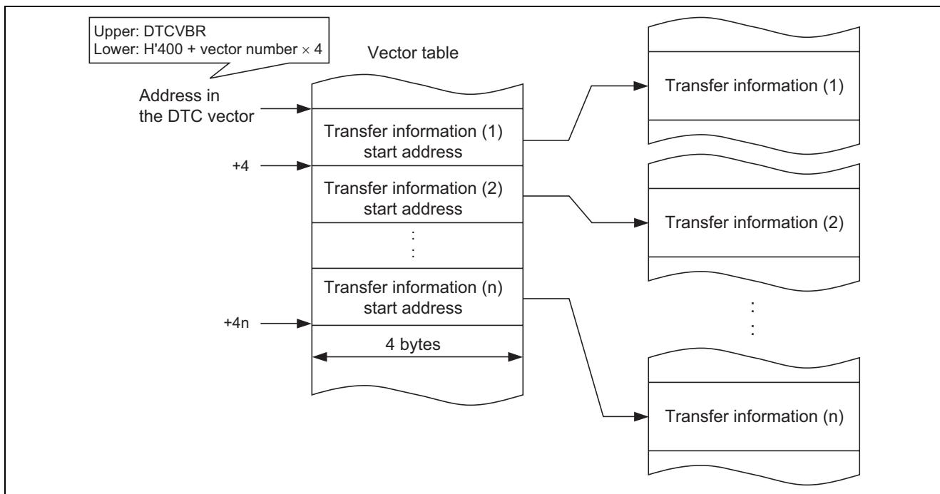
Figure 5 Correspondence between DTC Vector Addresses and Transfer Information
