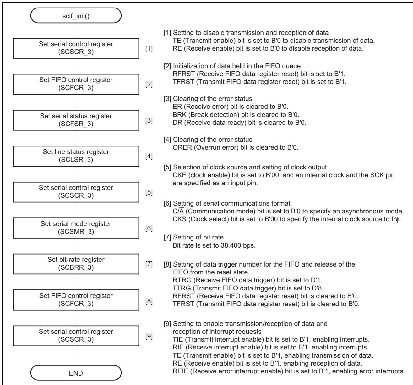
Figure 12 Flow for Initialization of Data Transmission and Reception in Asynchronous Mode
