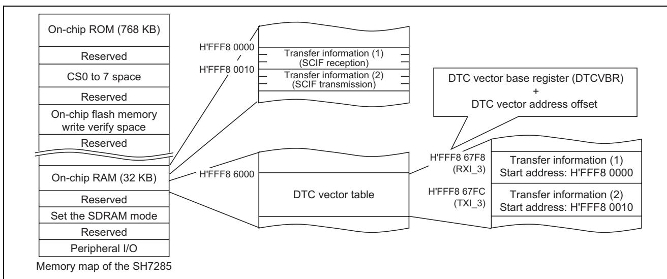
**Figure 6 Image of Arrangement of Transfer Information in Memory**
