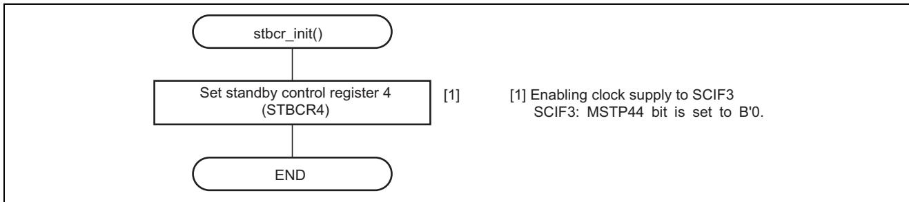
**Figure 9 Flow of Setting for Release from Module-Standby Mode**
