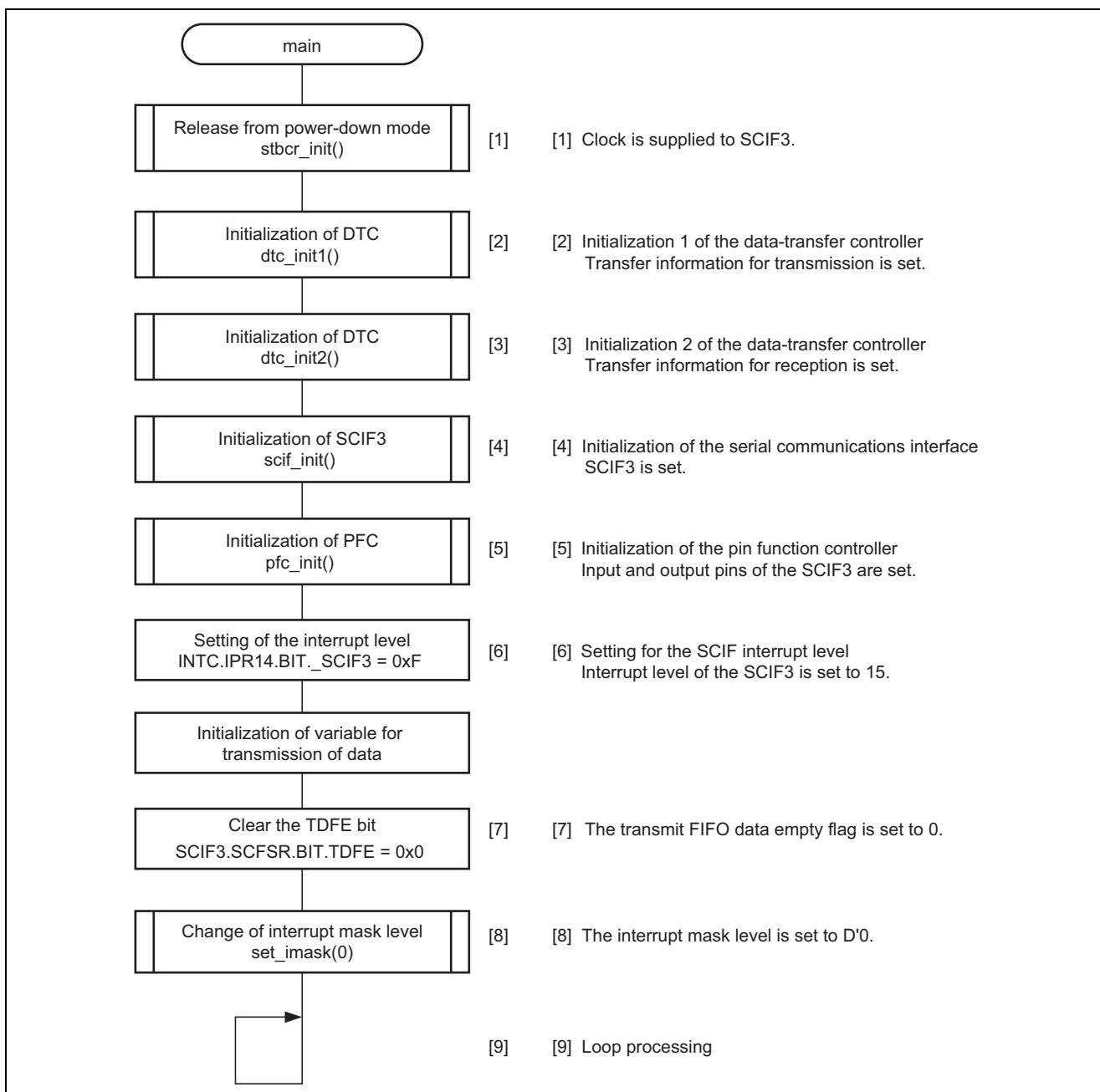
Figure 8 Flow of Processing by the Sample Program
