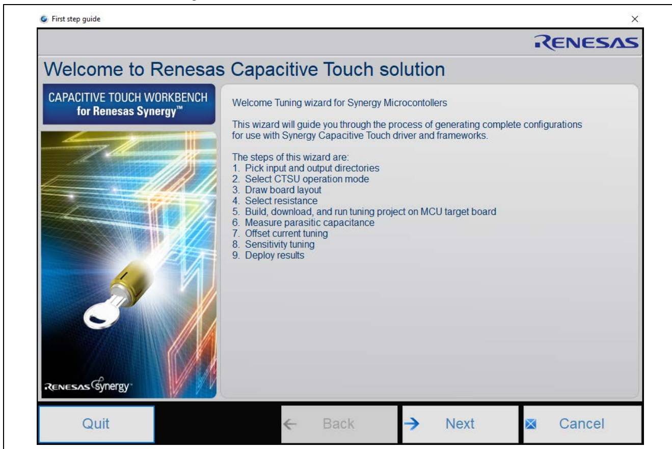
Figure 7. Major steps in tuning with CTW for Synergy
