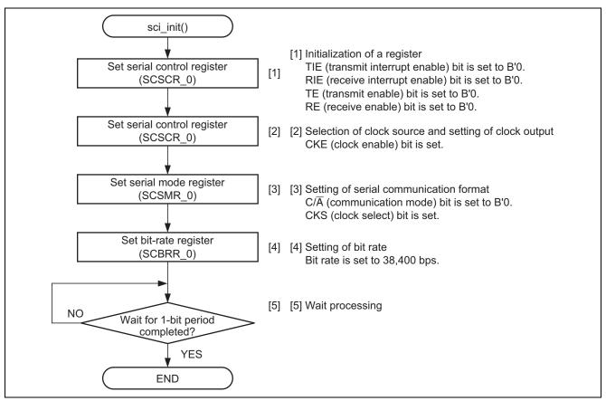
Figure 7 Flow for Initialization of Data Transmission in Asynchronous Mode
