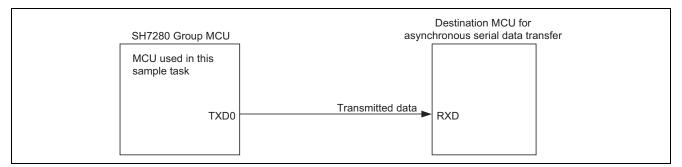
Figure 1 Connection Example for Transmission by the SCI in Asynchronous Mode
