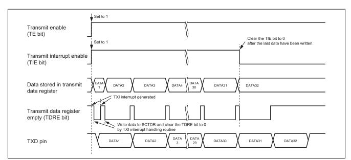
Figure 3 Operations for Data Transmission
