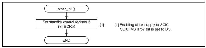
Figure 5 Flow of Settings for Release from Module-Standby Mode
