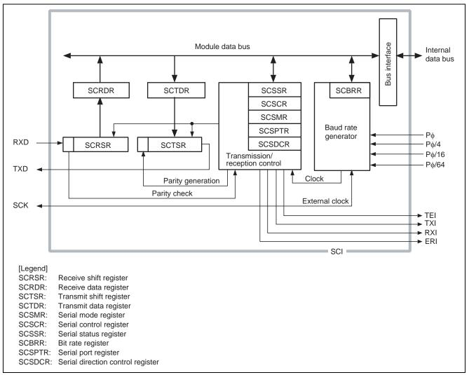
Figure 2 Block Diagram of the SCI
