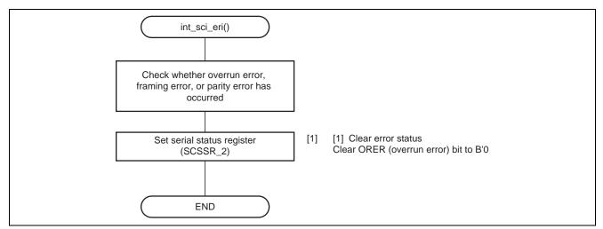
Figure 10 Flow for Handling Receive Error Interrupts in Clock Synchronous Mode
