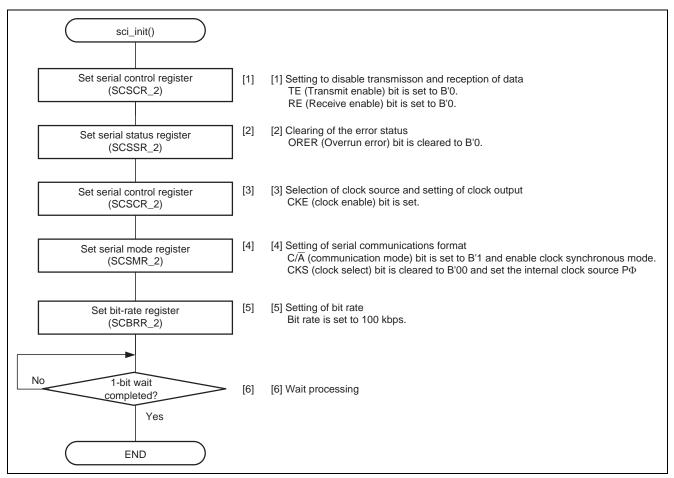
Figure 6 Flow for Initialization of Data Transmission and Reception in Clock Synchronous Mode
