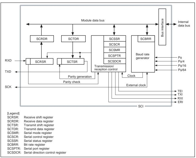
Figure 2 Block Diagram of the SCI
