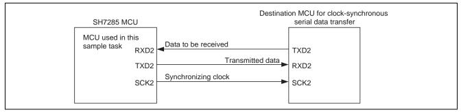
Figure 1 Connection Example for Transmission and Reception by the SCI
