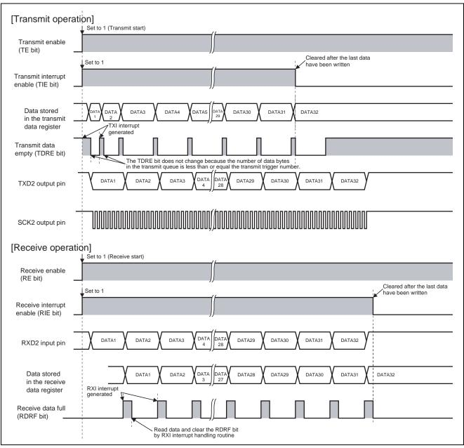
Figure 3 Operations for Data Transmission and Reception
