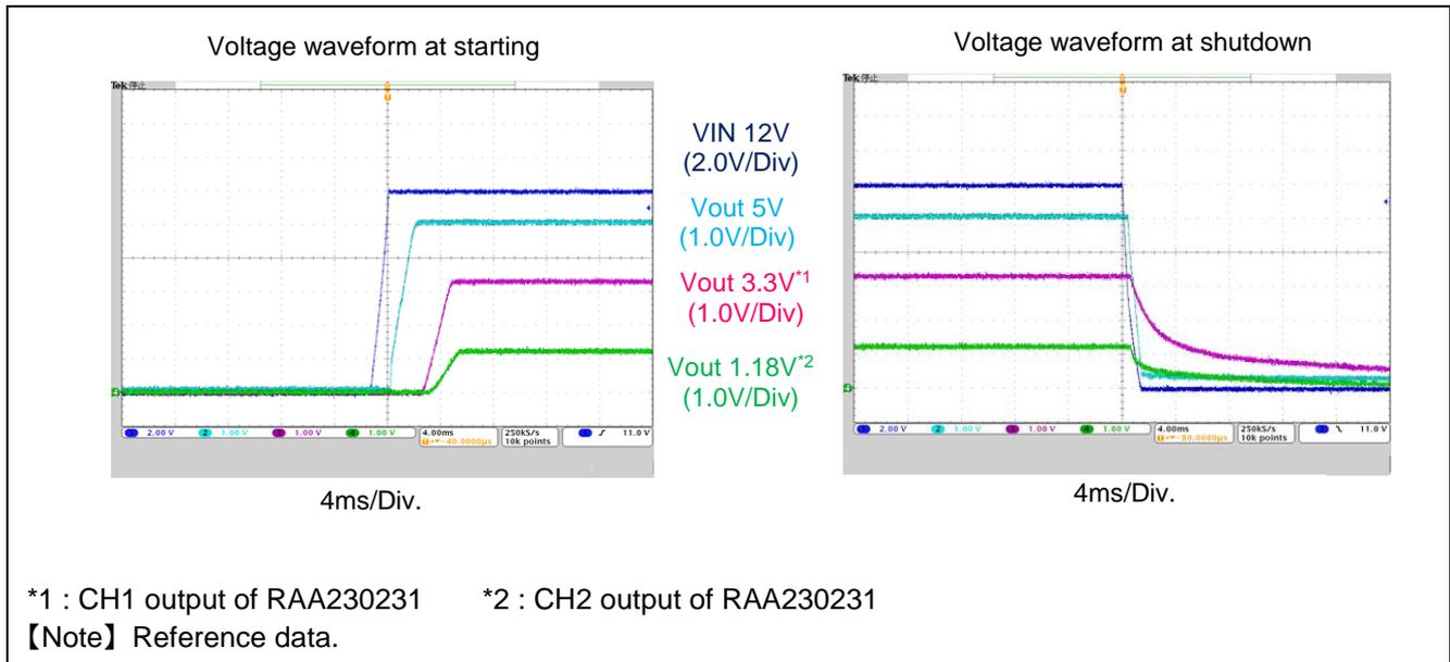
Fig2 Voltage waveform at starting and shutdown on GR-Peach
