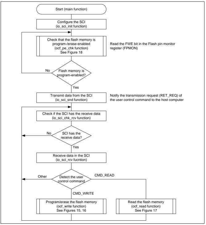
Figure 14 Main Processing Flow Chart
