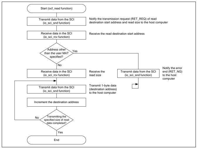
Figure 17 Reading the Flash Memory
