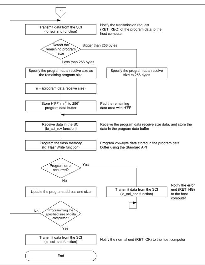
Figure 16 Programming/Erasing the Flash Memory (2/2)
