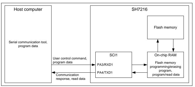
**Figure 1 System Configuration**
