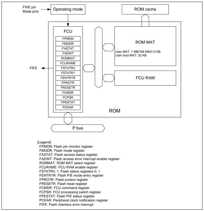
Figure 3 Flash Memory Block Diagram
