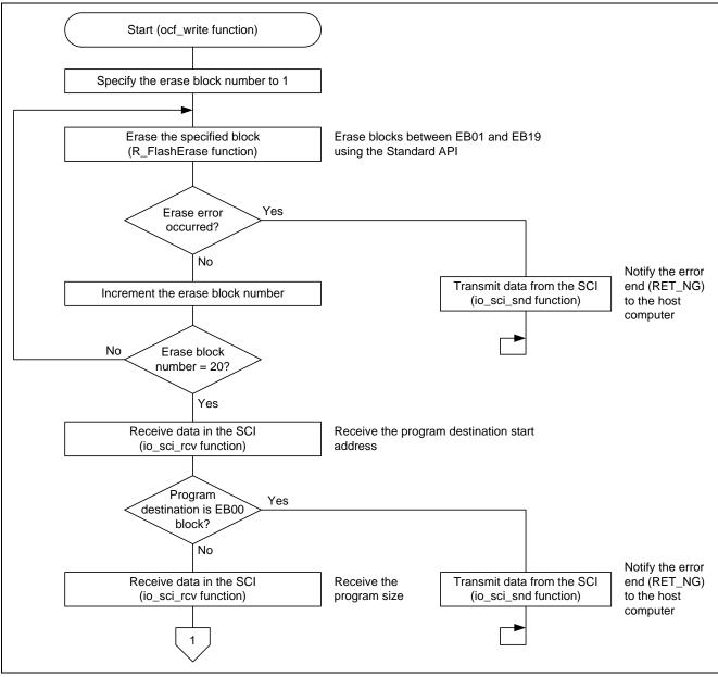
Figure 15 Programming/Erasing the Flash Memory (1/2)
