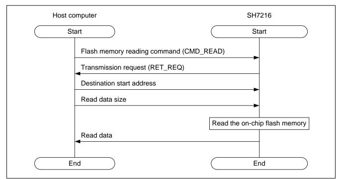
Figure 13 Communication Command Sequence When Reading the Flash Memory
