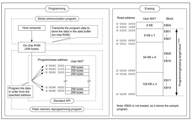
Figure 10 Programming and Erasing the Flash Memory
