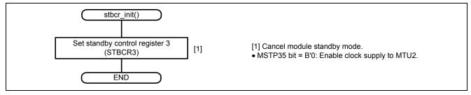
Figure 12 Initialization: Release from Standby
