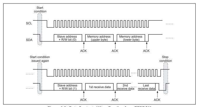
Figure 2.5 Data Contents When Reading from EEPROM
