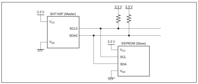
Figure 1.1 Connection of EEPROM to SH7145F
