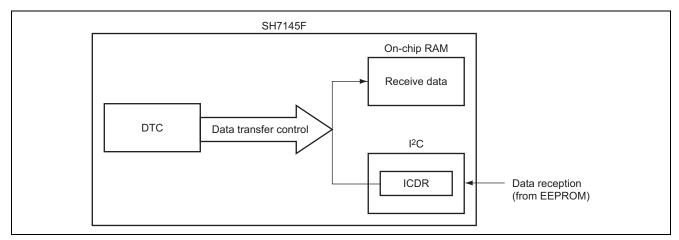
Figure 2.2 Data Transfer by DTC
