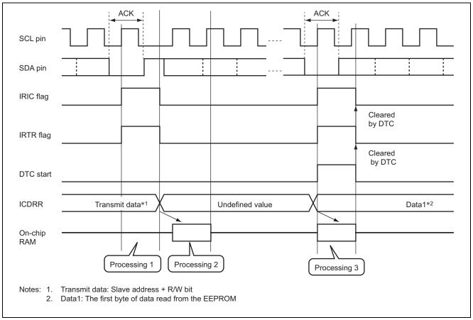
Figure 2.6 Operation When Data Read from EEPROM Starts
