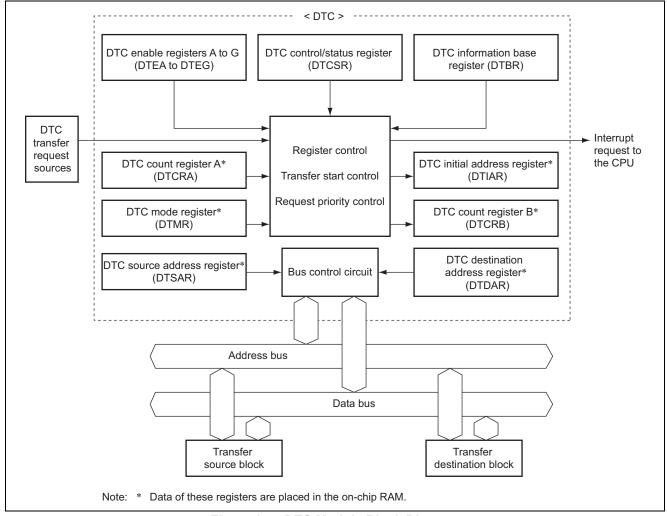
Figure 2.4 DTC Module Block Diagram
