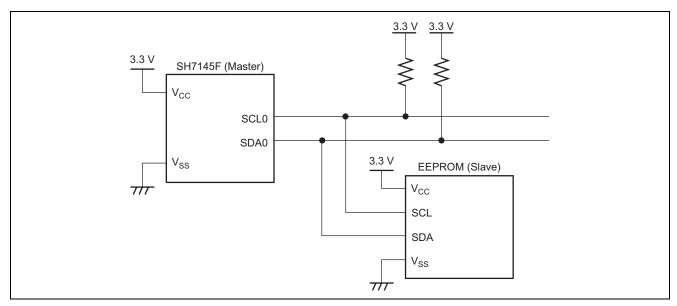
Figure 2.1 Connection of EEPROM to SH7145F
