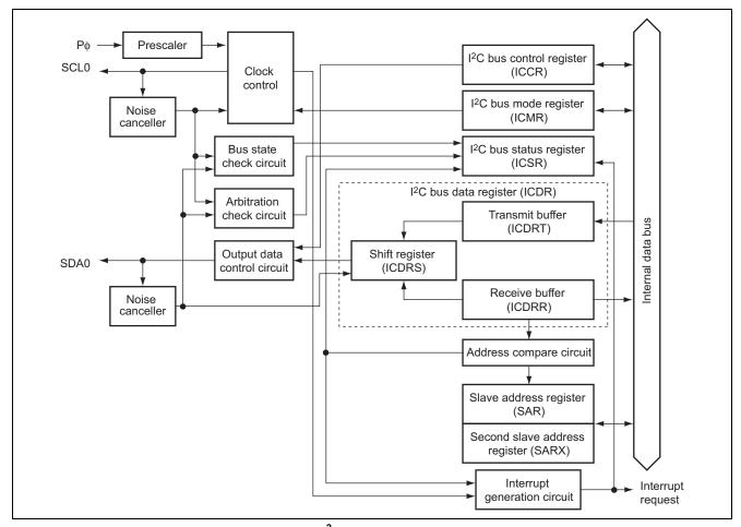
Figure 1.3 I<sup>2</sup>C Module Block Diagram
