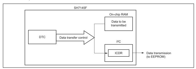
Figure 1.2 Data Transfer by DTC
