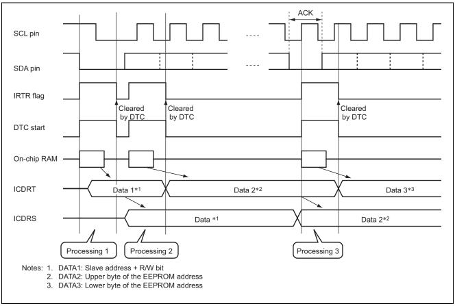
Figure 1.6 Operation When Data Write to EEPROM Starts
