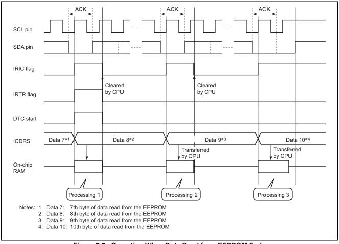
Figure 2.7 Operation When Data Read from EEPROM Ends
