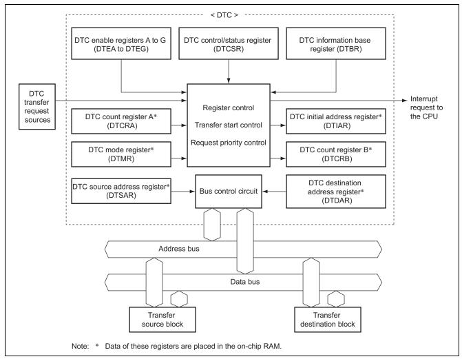
Figure 1.4 DTC Module Block Diagram
