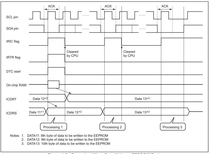
Figure 1.7 Operation When Data Write to EEPROM Ends
