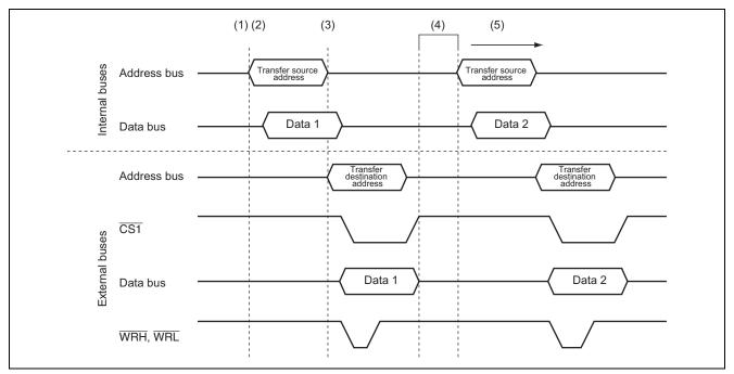
Figure 3 Operation by Direct Address Transfer in Dual Address Mode
