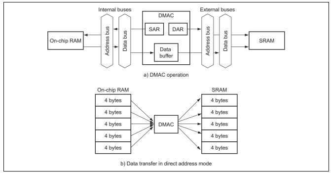
Figure 1 illustrates data transfer by the DMAC; table 1 shows the DMAC settings.
