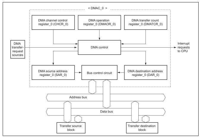
Figure 2 DMAC Block Diagram (ch0)
