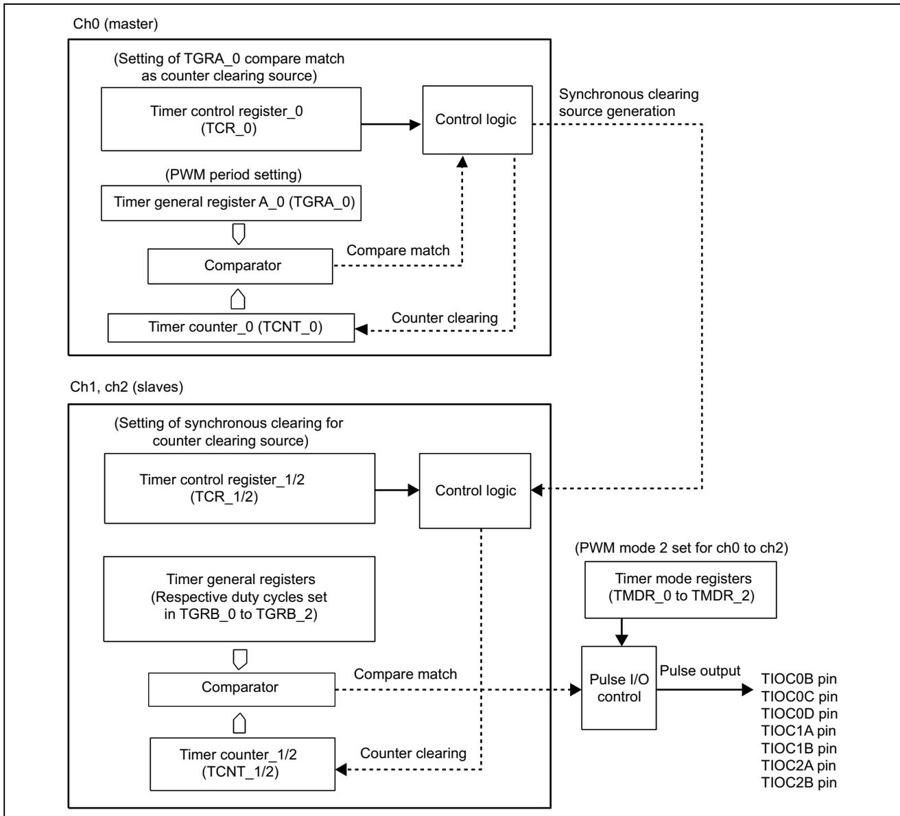
Figure 2 Block Diagram of Synchronous Clearing
