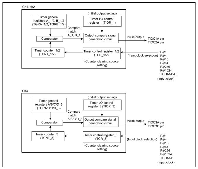
Figure 2 Block Diagram of MTU/ch1, ch2, ch3
