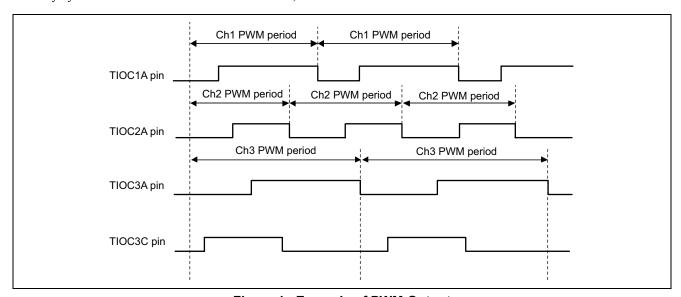
Figure 1 Example of PWM Output
