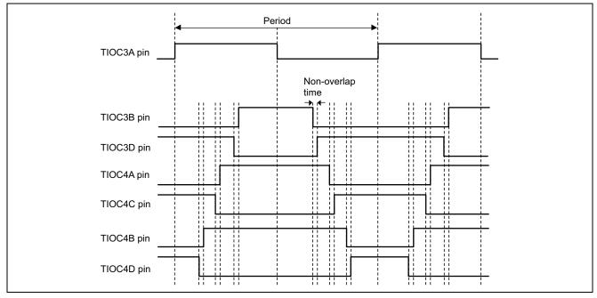
Figure 1 Complementary PWM 3-Phase Output Waveforms
