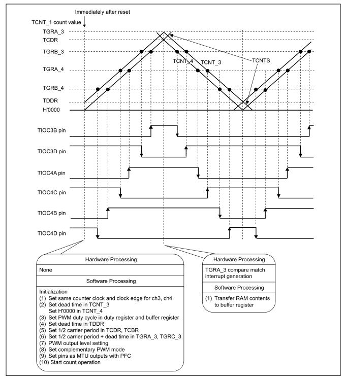
Figure 6 Principles of Operation of PWM Waveforms
