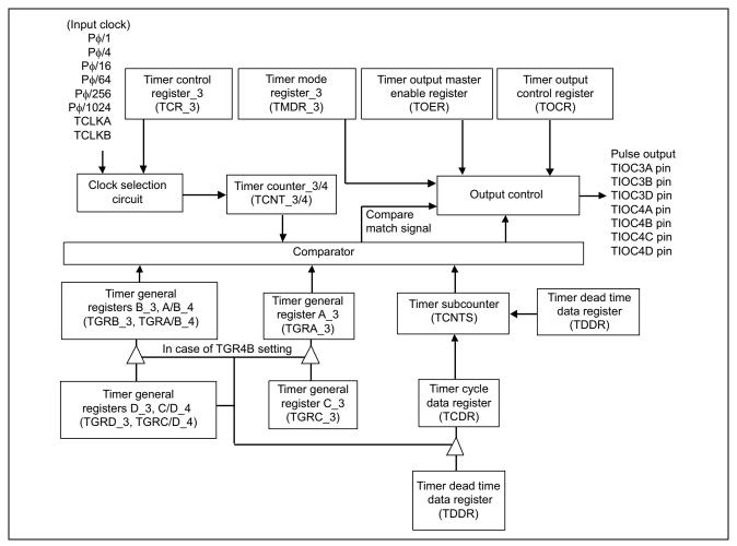
Figure 2 Block Diagram of MTU/ch3, ch4
