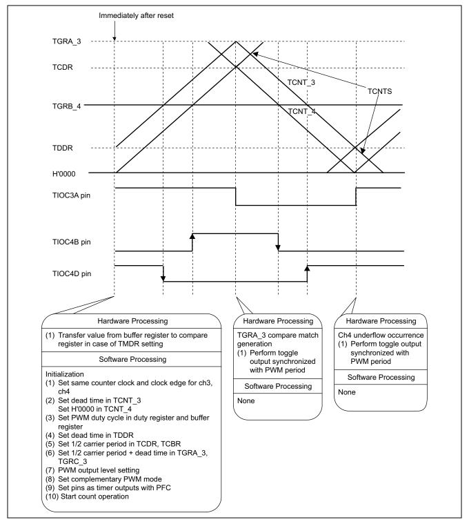
Figure 7 Principles of Operation of Toggle Waveform Output Synchronized with PWM Period
