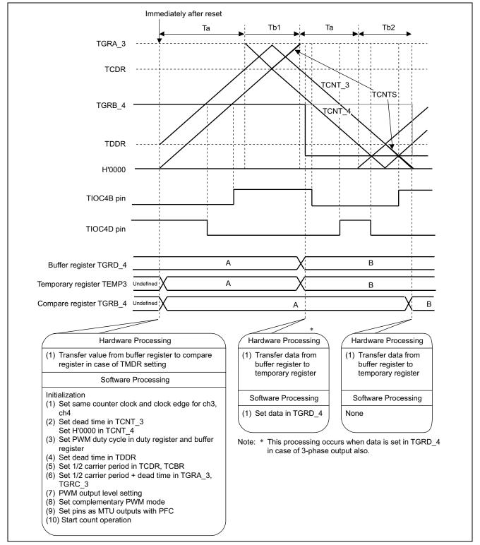
Figure 5 Principles of Operation of Complementary PWM Single-Phase Waveform Output
