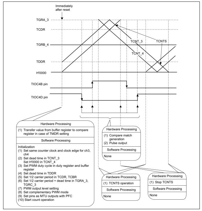
Figure 3 Principles of Operation of Complementary PWM Single-Phase Waveform Output
