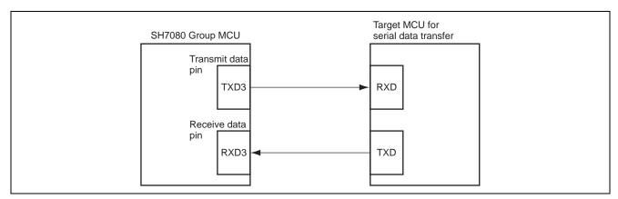
Figure 1 Asynchronous Serial Data Transmission and Reception with FIFO
