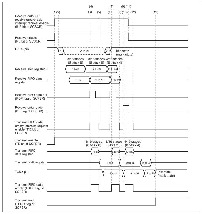
Figure 3 Principles of Operation
