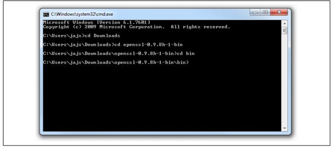
Figure 5 Navigation to openssl binary folder
