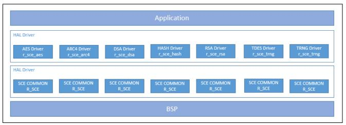
Figure 1 SCE HAL Module Block Diagram
