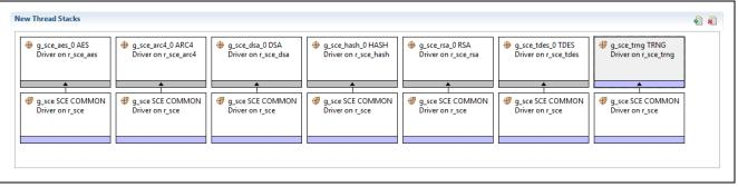
Figure 2 SCE HAL Module Stack (AES, ARC, DSA, HASH, RSA, TDES, and TRNG included)
