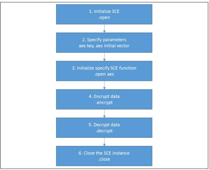
Figure 3 Flow Diagram of a Typical Cryptography Application
