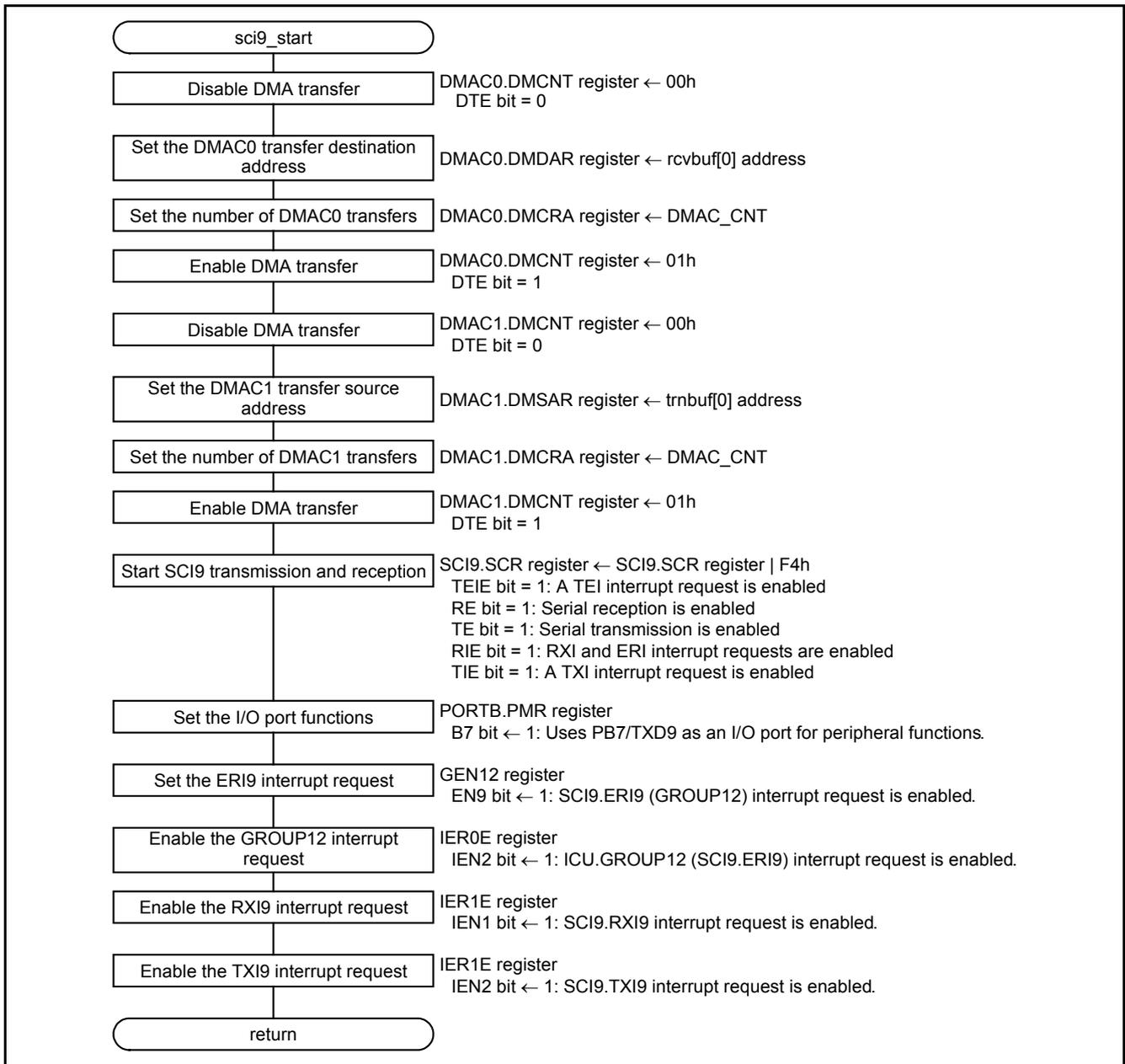
Figure 5.9 SCI9 Transmission/Reception Start
