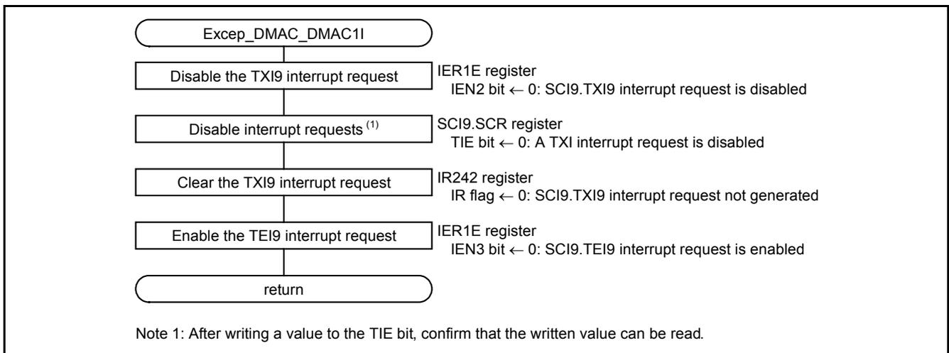
Figure 5.11 DMAC1 Transfer End Interrupt Handling
