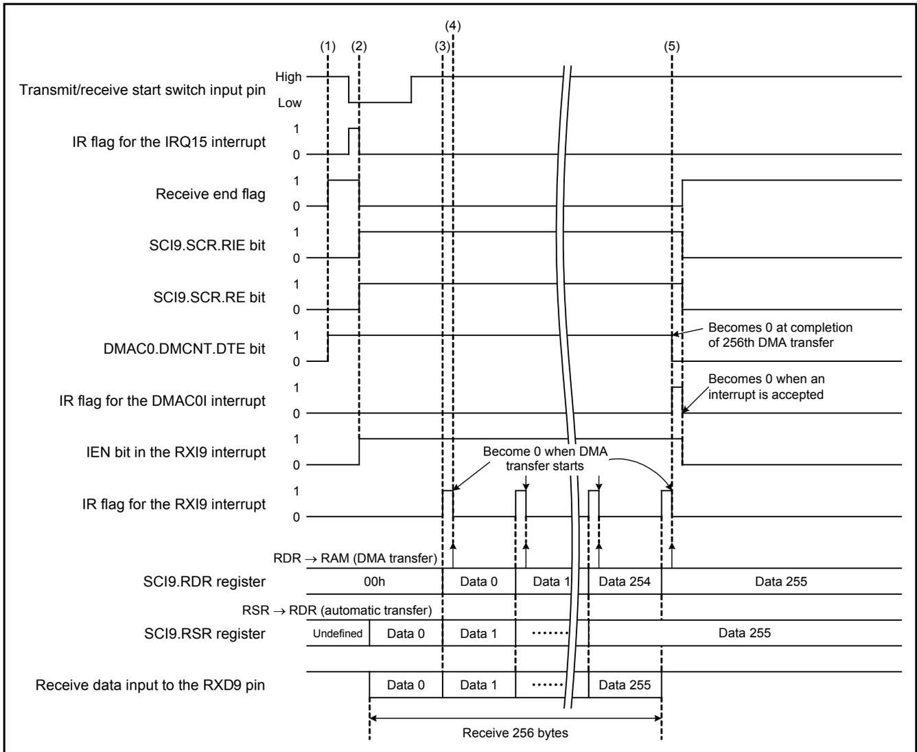
Figure 5.2 Timing Diagram When Receiving Data
