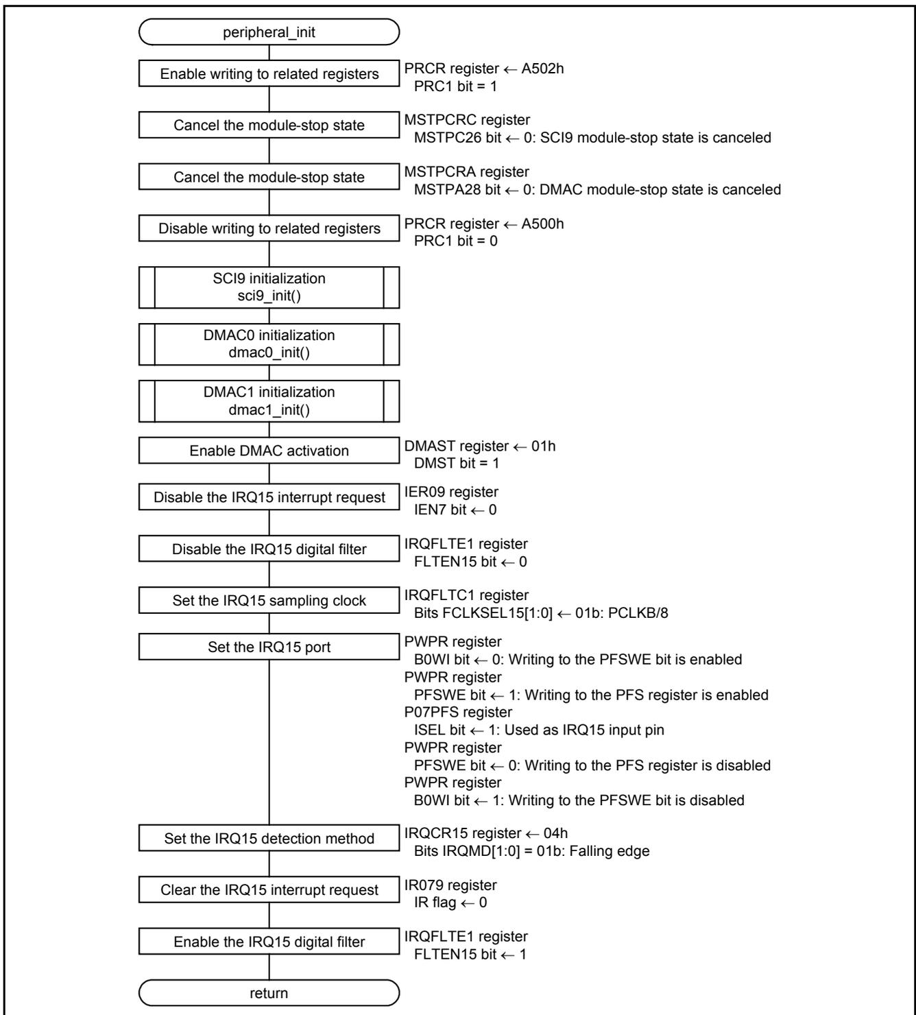
Figure 5.5 Peripheral Function Initialization
