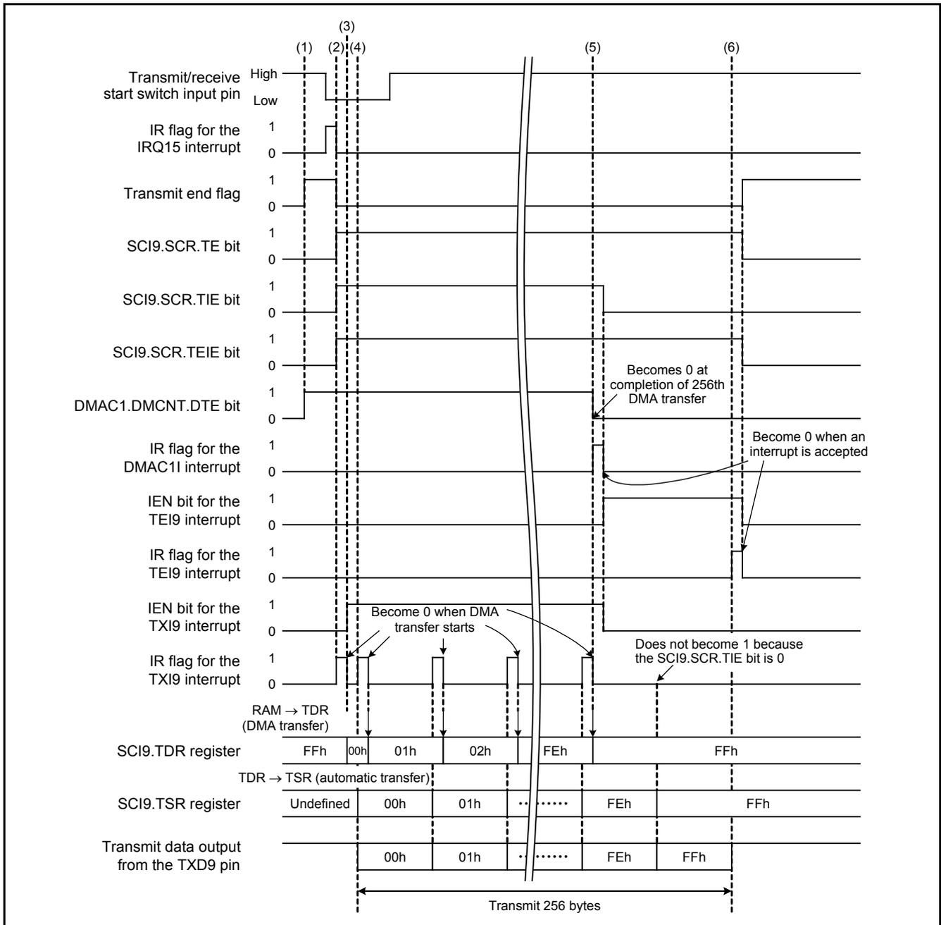
Figure 5.1 Timing Diagram When Transmitting Data
