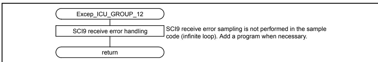
Figure 5.13 Group 12 Interrupt Handling (SCI9 Receive Error Interrupt)
