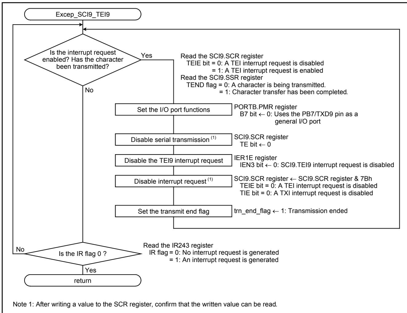
Figure 5.12 SCI9 Transmit End Interrupt Handling
