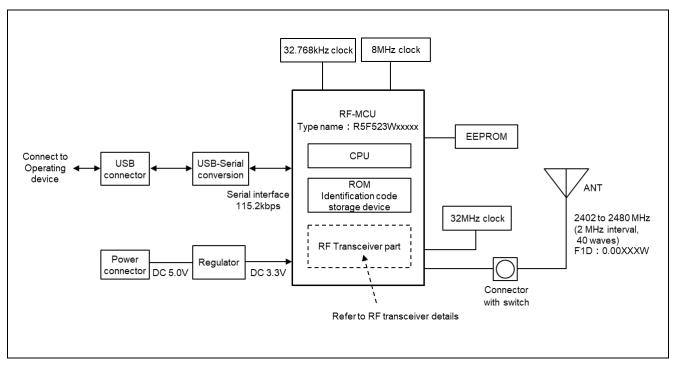
Figure 2-1. Block diagram of radio equipment (Example)
