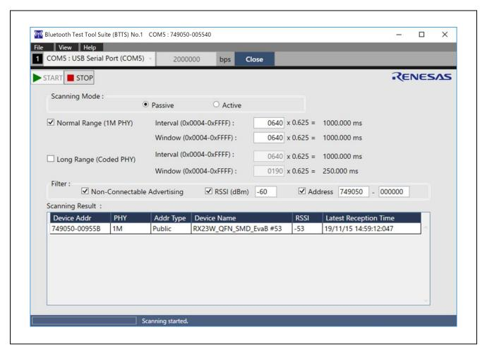
Figure 3-5. Scanning setting (receiving device side)
