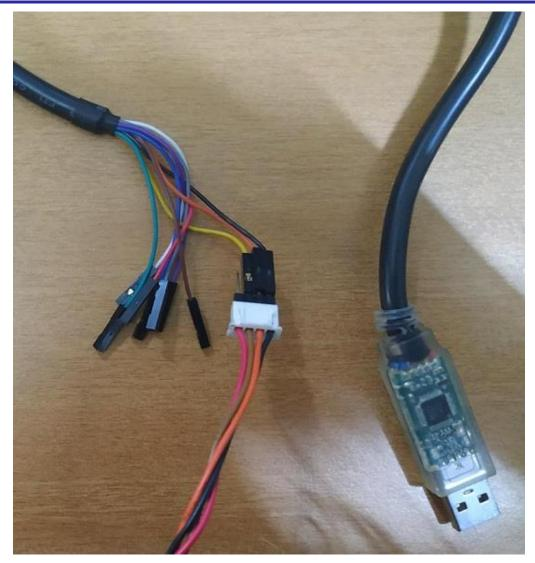
Figure 9 USB- Serial Cable
