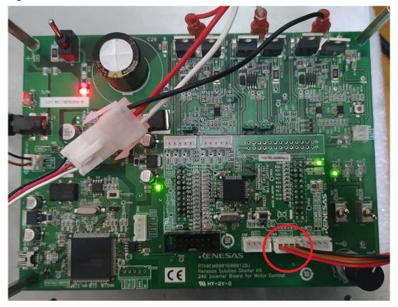
Figure 7 SCI connections of RX23T
