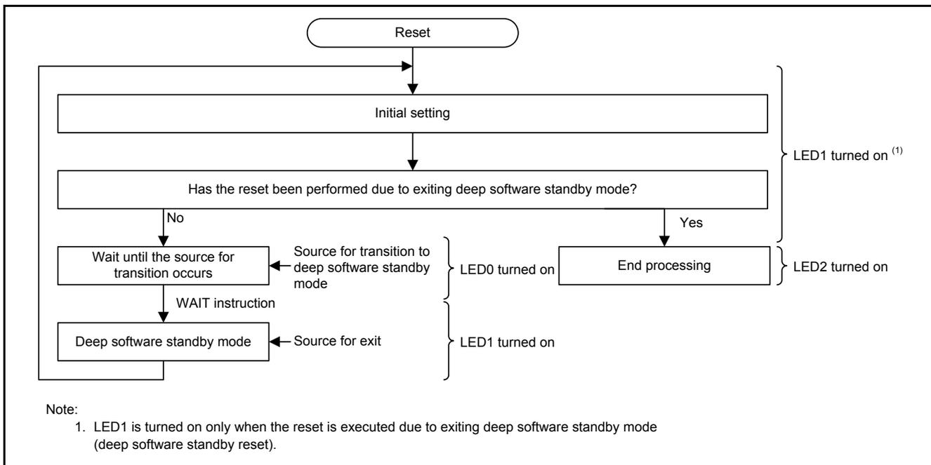
Figure 5.3 Operation Overview when Entering and Exiting Deep Software Standby Mode
