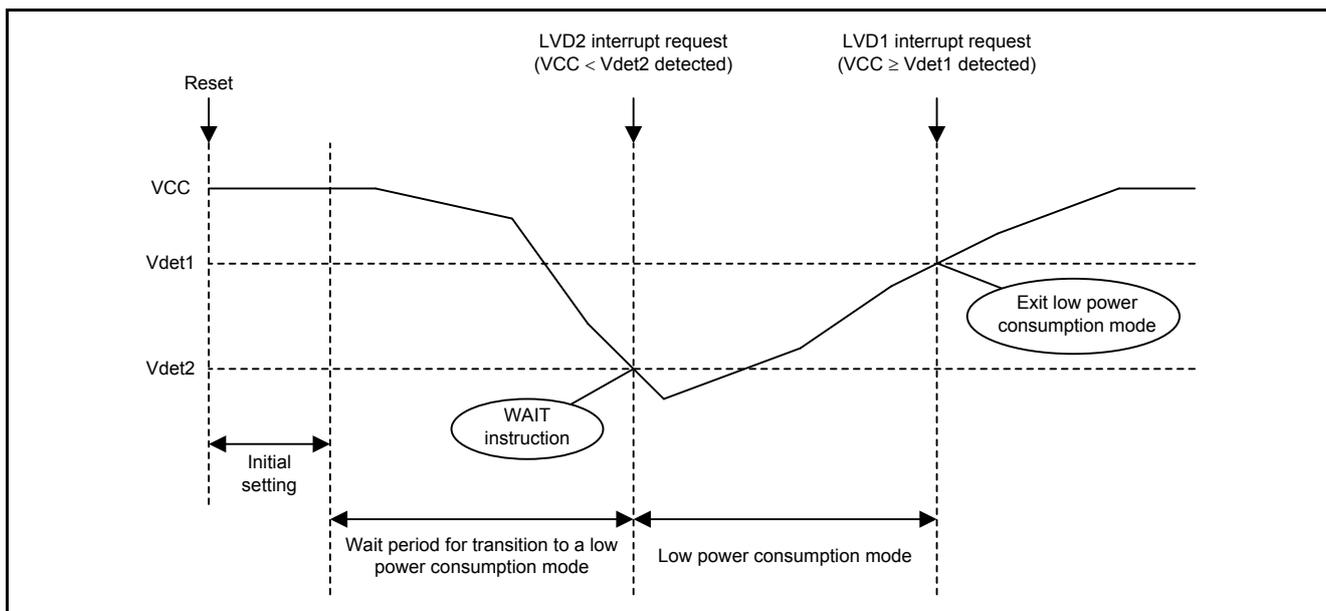
Figure 5.6 Timing of Entering and Exiting a Low Power Consumption Mode Using the LVD
