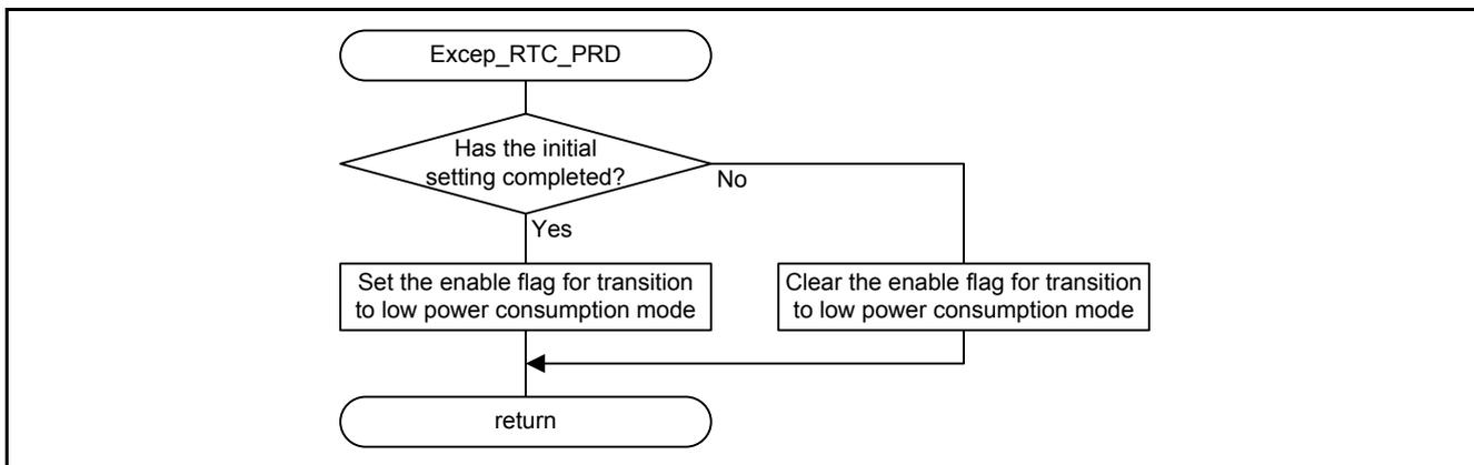
Figure 5.22 RTC.PRD Interrupt Handling
