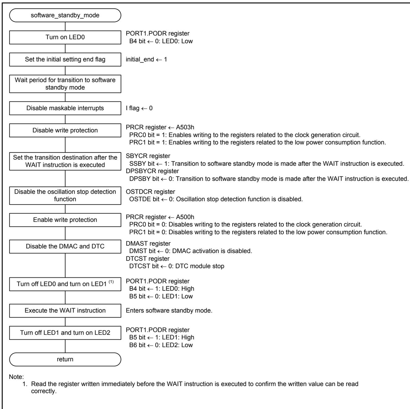
Figure 5.11 Transition to Software Standby Mode
