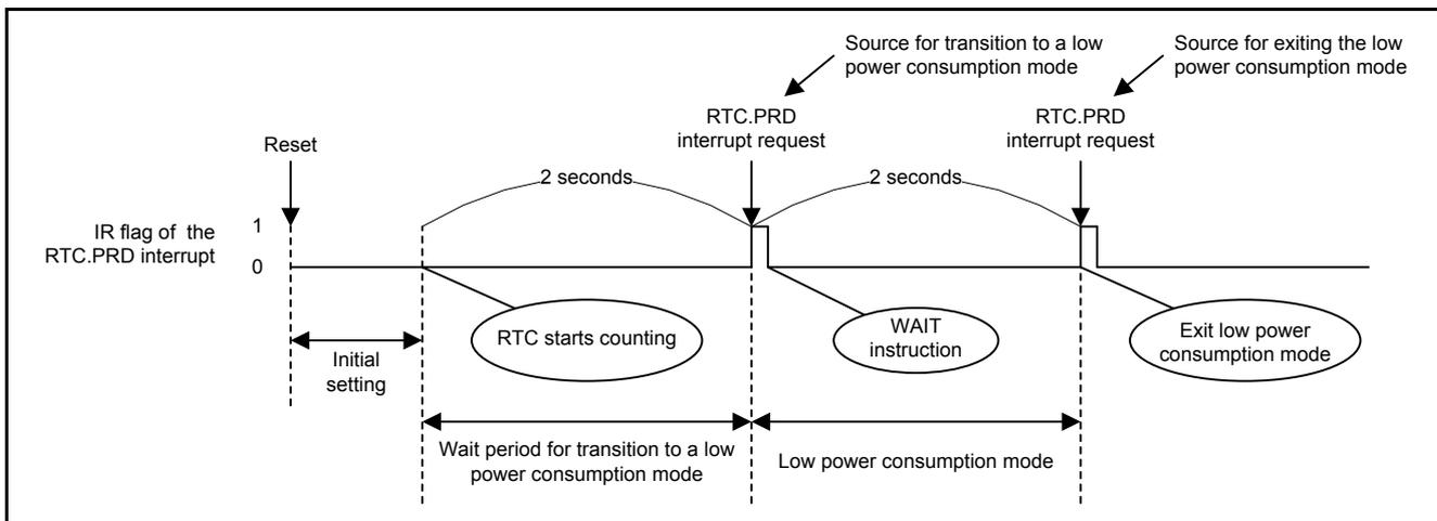
**Figure 5.5 Timing of Entering and Exiting a Low Power Consumption Mode Using the RTC**
