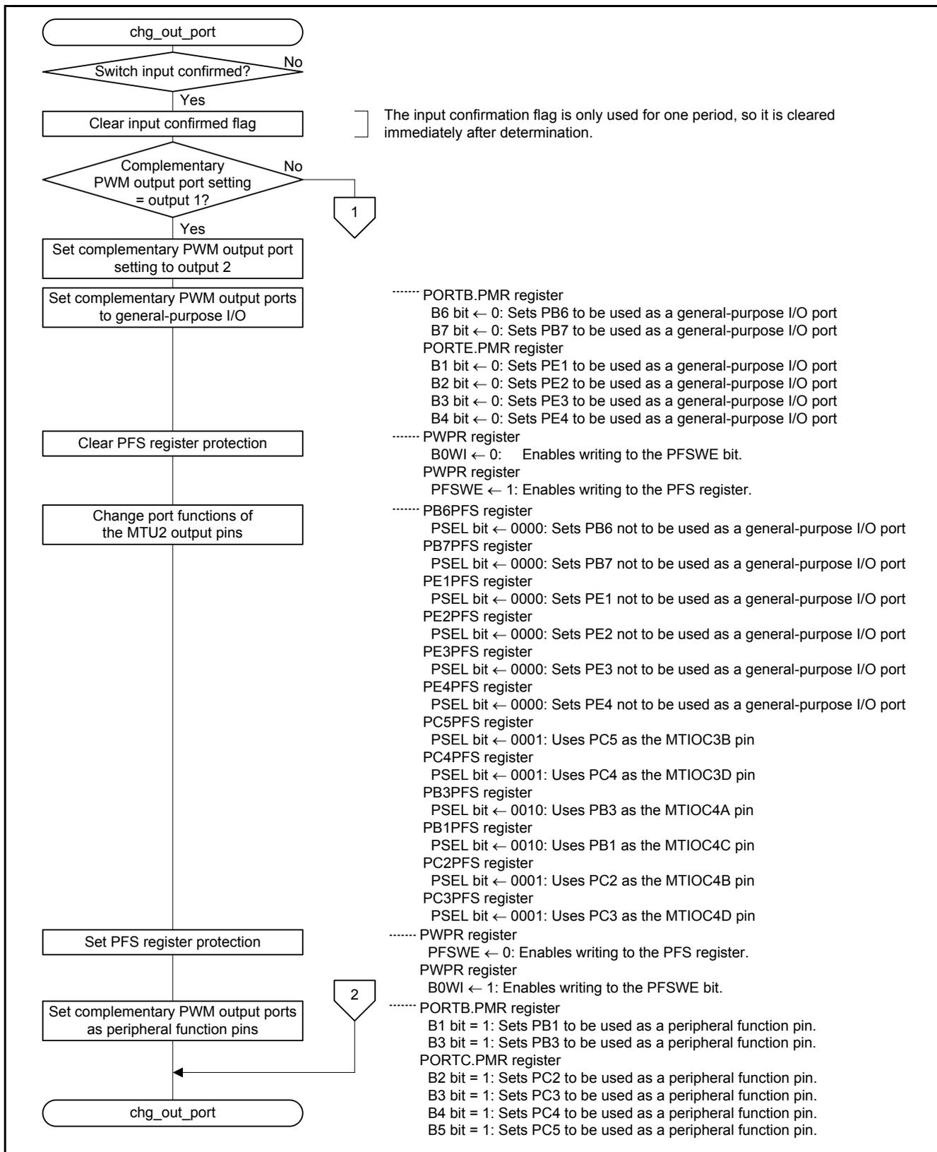
Figure 5.10 Complementary PWM Output Port Switching (1/2)
