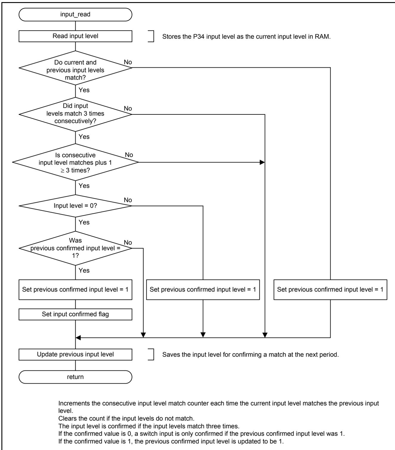
Figure 5.9 Reading Switch Input
