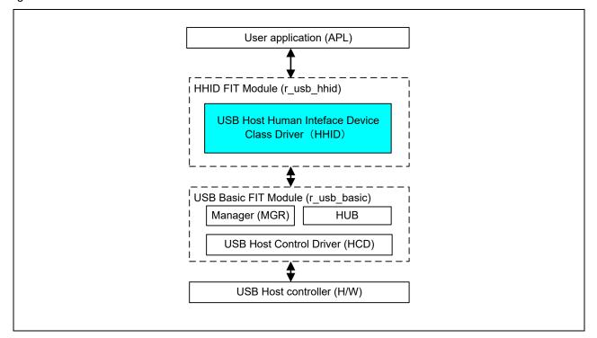
Figure 2-1 Software Module Structure
