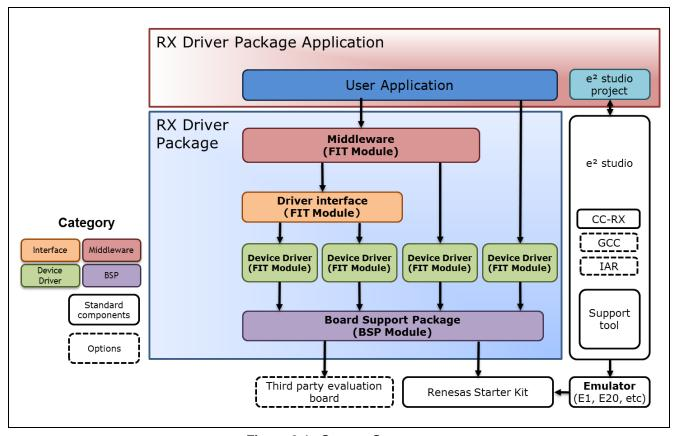
Figure 2-1 System Structure
