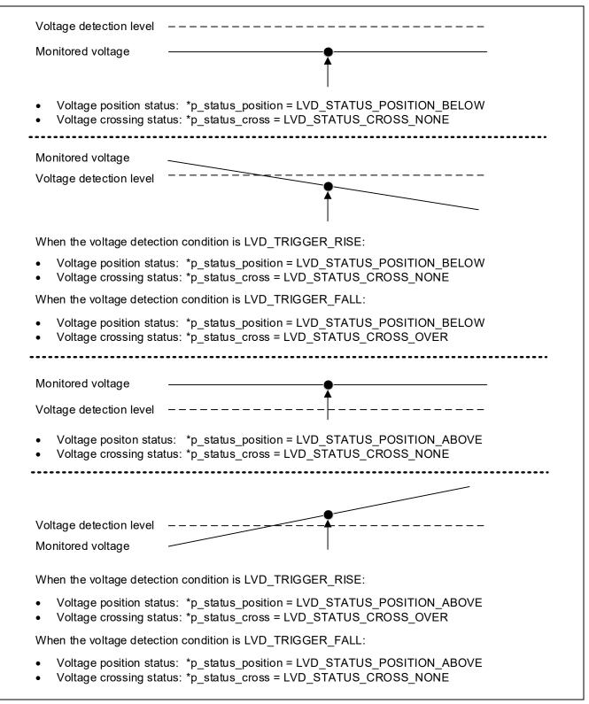
Figure 3.1 Monitored Voltage Status Relative to the Voltage Detection Level and the LVD Status
