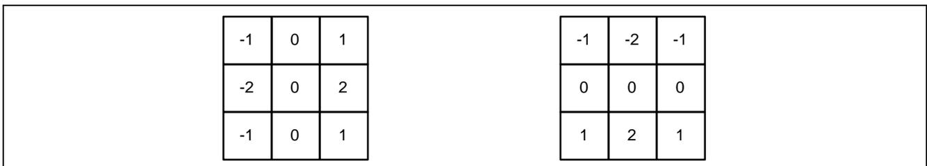
**Figure 6 Sobel Filter Masks (Left: Horizontal, Right: Vertical)**
