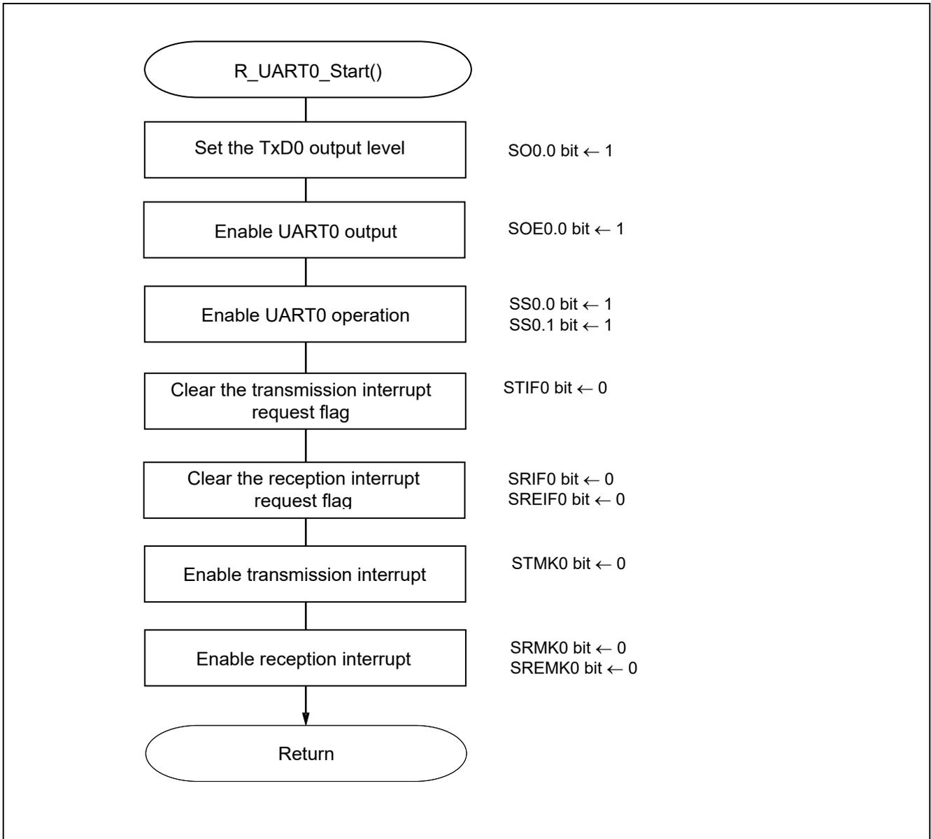
**Figure 5.15 UART0 Operation Start Function**
