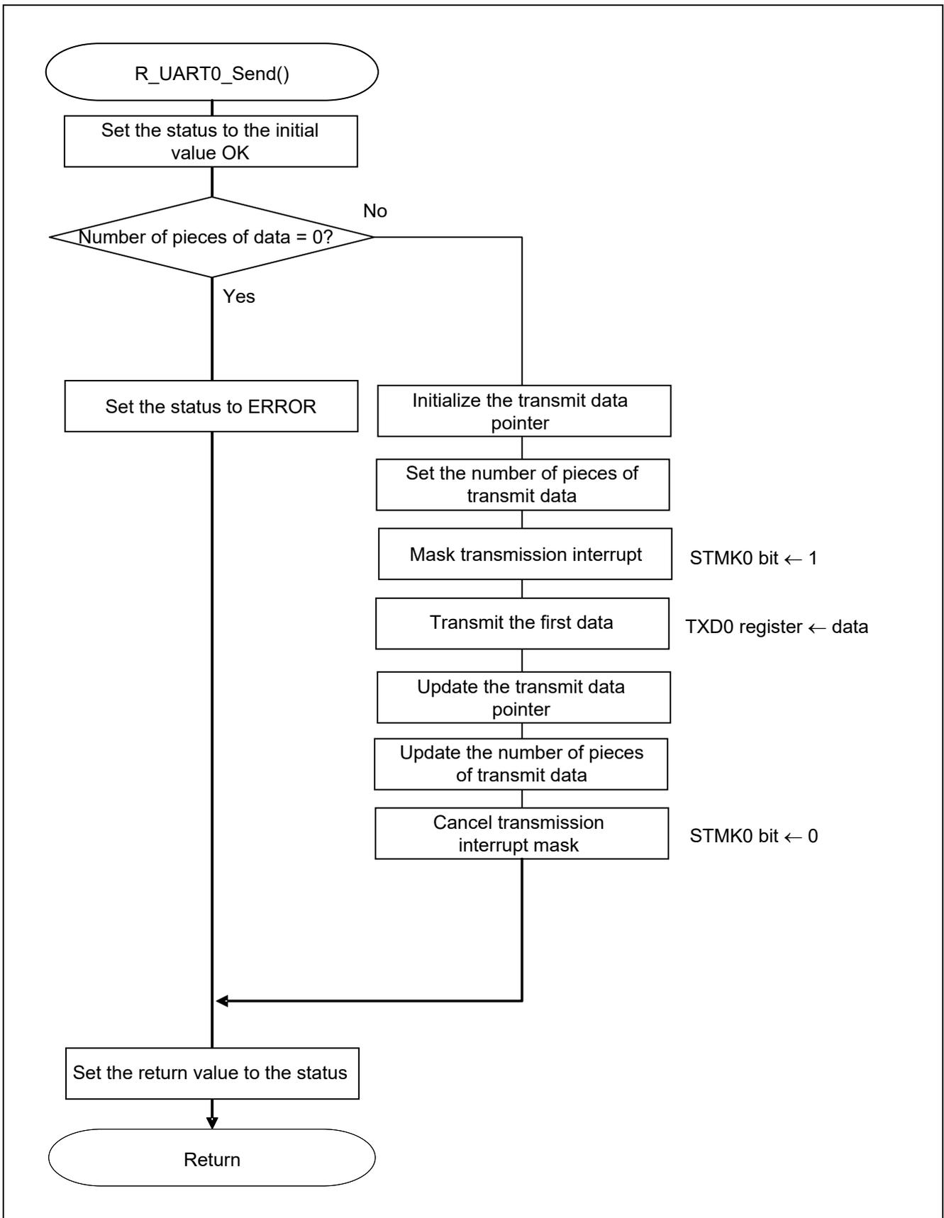
Figure 5.18 UART0 Data Transmission Function
