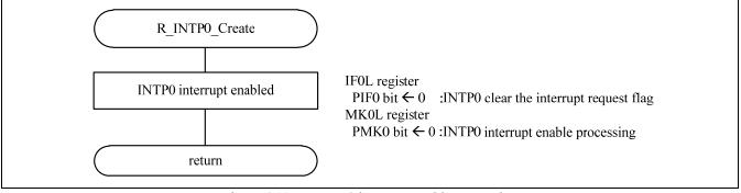
Figure 4.11 INTP0 interrupt enable processing
