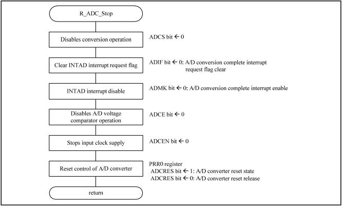
Figure 4.22 A/D converter stop processing
