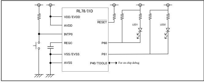
Figure 3.1 Hardware structure
