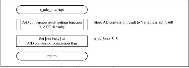
Figure 4.27 A/D conversion complete interrupt processing
