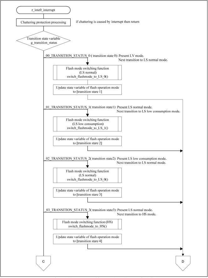
Figure 4.24 External interrupt (INTP0) processing(1/2)
