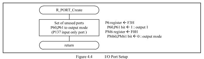
Caution: Provide proper treatment for unused pins so that their electrical specifications are observed. Connect each of any unused input-only ports to VDD or Vss via a separate resistor.
