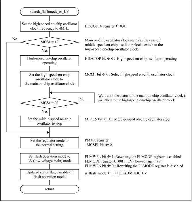
Figure 4.14 Flash operation switching (LV) processing
