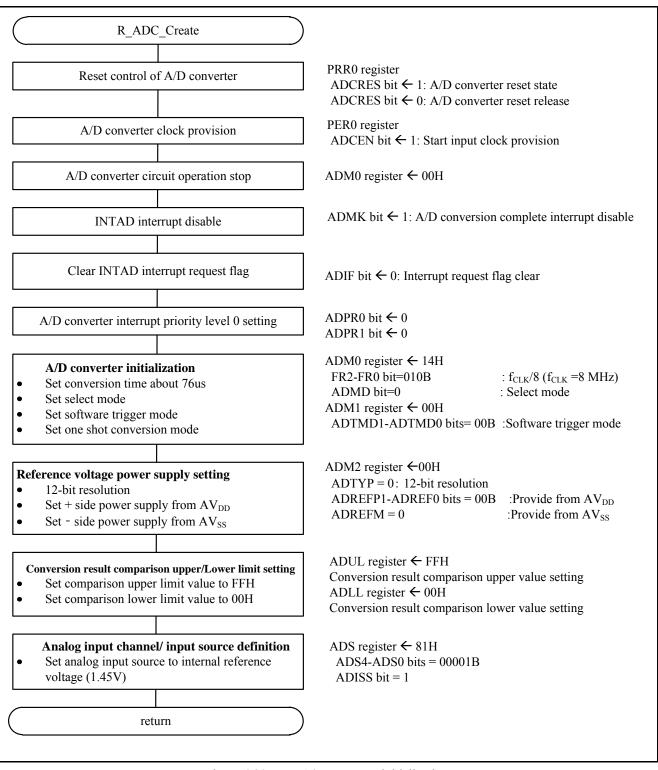
Figure 4.20 A/D converter initialization
