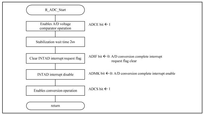
Figure 4.21 A/D conversion operation start processing
