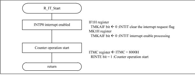
Figure 4.12 12-bit interval timer start processing
