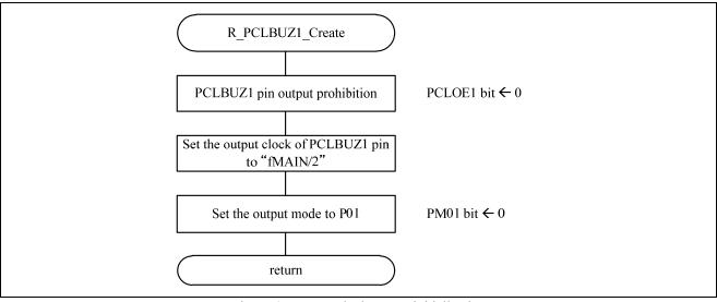
Figure 4.7 clock output initialization
