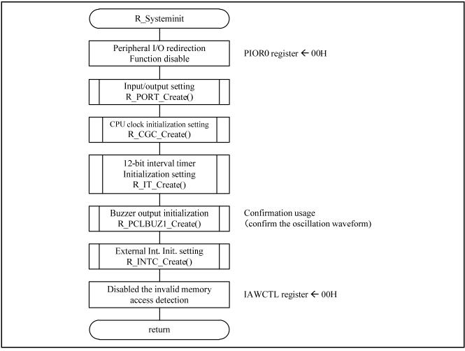
Figure 4.3 Peripheral function initialization
