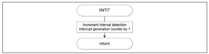
Figure 5.74 12-bit Interval Timer Interrupt Servicing
