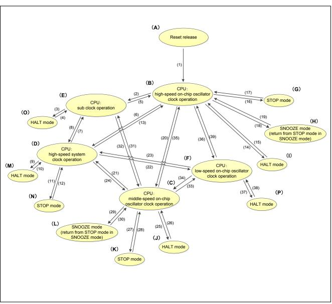
Figure 1.1 Operating Mode Status Transition Diagram
