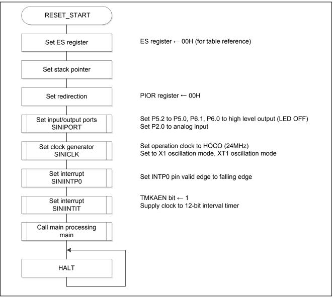
Figure 5.3 CPU Initialization Function
