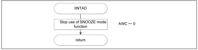
Figure 5.75 A/D Conversion Completion Interrupt Servicing
