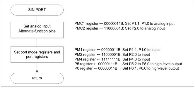
Figure 5.4 Input/Output Port Settings
