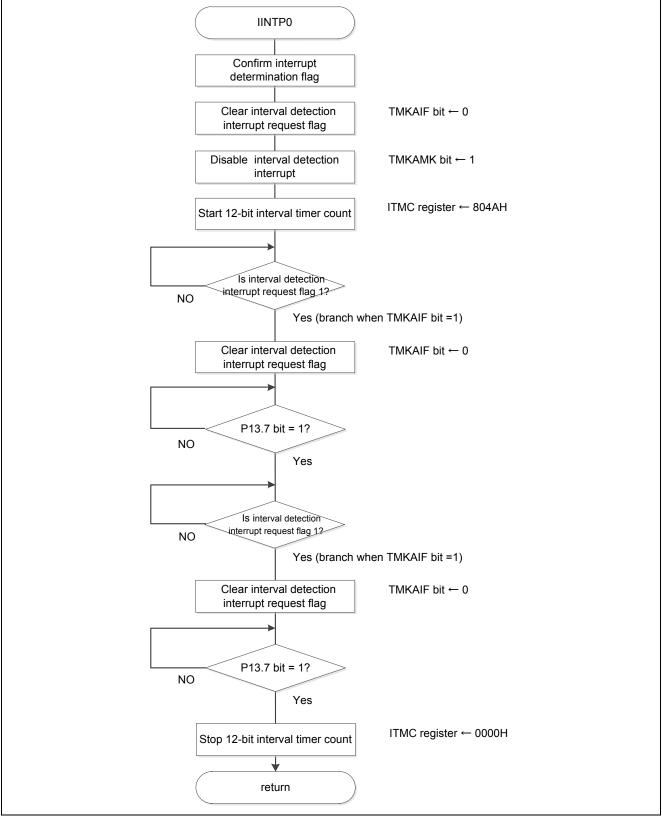
Figure 5.73 External Interrupt Servicing
