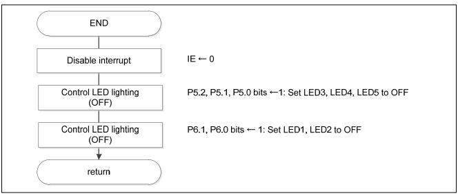
Figure 5.72 Status Transition End Processing
