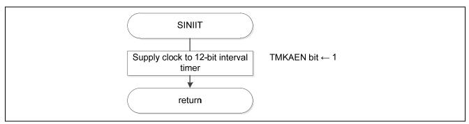
Figure 5.7 12-bit Interval Timer Setting
