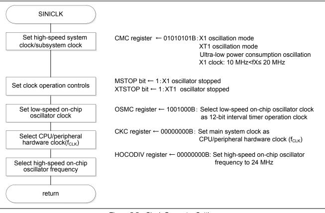
Figure 5.5 Clock Generator Setting
