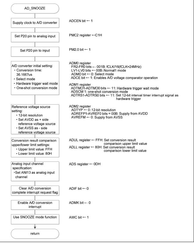
Figure 5.38 A/D Converter Setting
