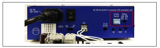
Step 5. Connect power cable to AC/DC 2-Converter unit and turn on the power by ON-OFF switch. RED LED (STATUS) is light on when the unit is on.
