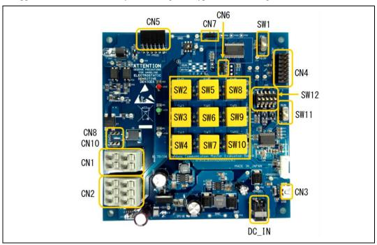
To evaluate the communication master board, use provided onboard connectors and switches for respective interface. Use SW11 and SW12 to set run mode for operation or set to write mode for reprogramming the board.
