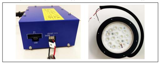
**Step 3.** Set "Normal operation mode": Configuration Switch 1, 2, 3, and 4 to OFF position and Debug Switch to RUN position.
