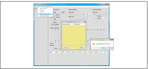
Step 8. Click "Start" button and prompt "DALI controller" message box. Click "OK" button and wait for completion of assigning the short address. Then click "Close" button after assigning the address.
