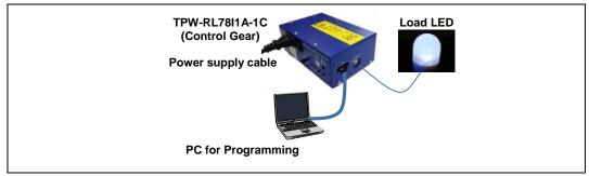
The demo unit comes with three operation modes: Normal Operation mode, OCD/Flash mode, and Virtual UART mode. You can select respective operation by Configuration Switch and Debug Switch setting as below.
