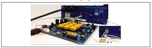
Step 4. Set "Normal operation mode" to AC/DC 2-Converter unit: Configuration Switch 1, 2, 3, and 4 to OFF position and Debug Switch to RUN position.
