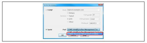
Step 6. Form "Setup" pulldown menu, select "Terminal". Then configure Terminal and click "OK" button.
