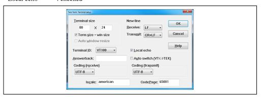
Step 7. Setup COM port setting form "Setup" pulldown menu and select "Serial port". Then configure serial port setting as below. Click "OK" button after configuration.
