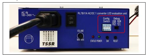
Step 4. Connect power cable to AC/DC 1-Converter unit and turn on the power by ON-OFF switch. Both RED LED (STATUS) and GREEN LED (POWER) are light on when the unit is on.
