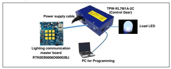
The demo unit offers three operation modes: Normal Operation mode, OCD/Flash mode, and Virtual UART mode. For operation, select one of the modes by using Configuration Switch and Debug Switch setting as below.
