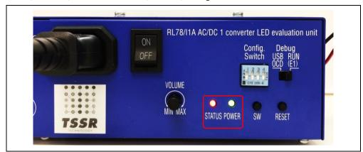
Step 5. Press SW switch to calibrate the newly attached LED module with AC/DC 1-Converter unit. If the LED module is within the limit of AC/DC 1-Converter unit, the RED LED will turn off. If not, it will blink to indicate the error. Press RESET switch to reset the AC/DC 1-Converter unit in case of error.
