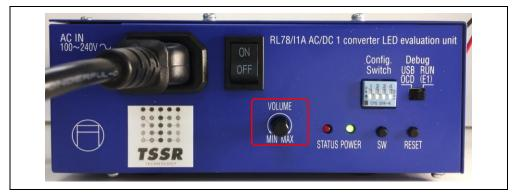
Below shows the working test setup of the AC/DC 1-Converter unit, which attached with LED module.
