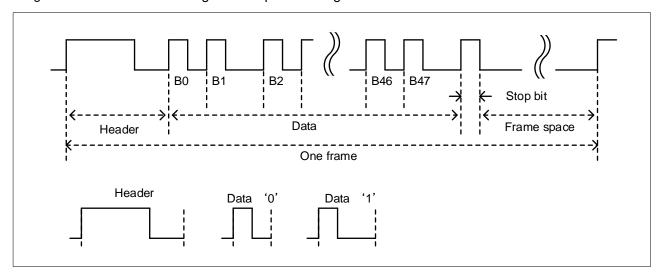
Table 1-3 shows the correspondence between remote control input signals and remote control signal data. When the fifth byte (B32 to B39 in Figure 1-2) of the received remote control signal data matches the signal data in Table 1-3, the application recognizes that the relevant channel button was pressed.
