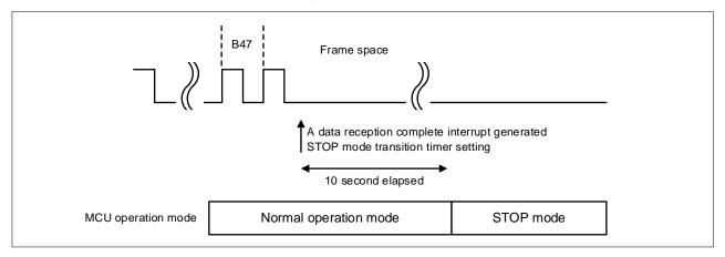
Figure 1-4 Remote Control Signal Reception State Transition Diagram
