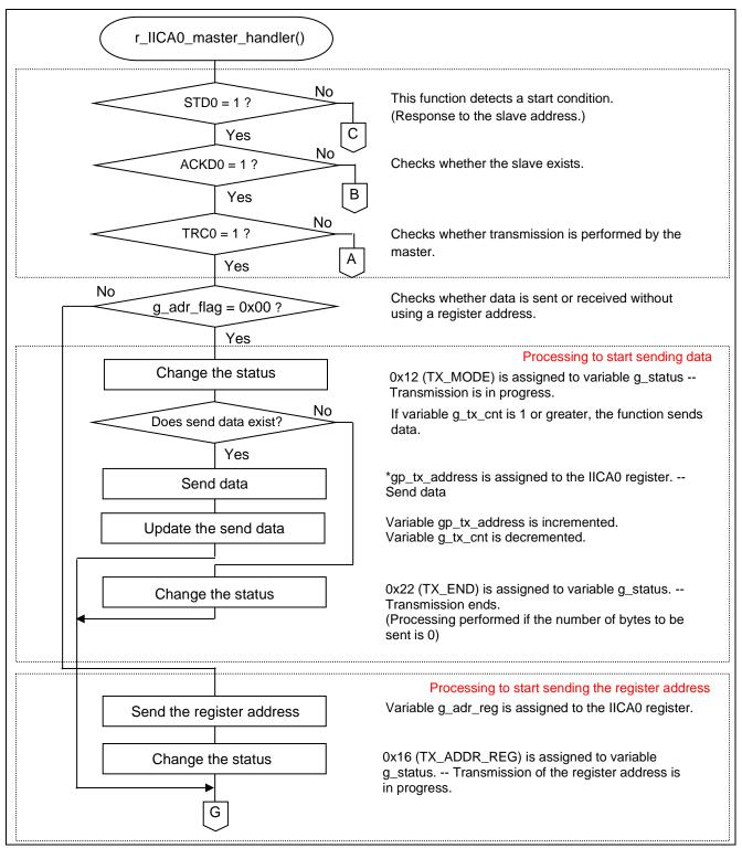
Figure 4-7 IICA0 Master Interrupt Processing Function (2/4)
