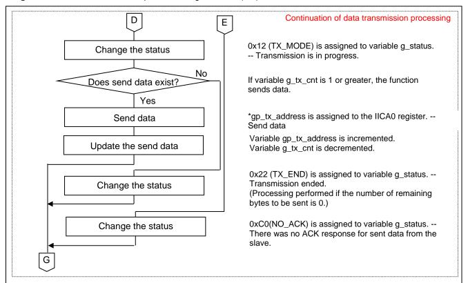
Figure 4-9 IICA0 Master Interrupt Processing Function (4/4)
