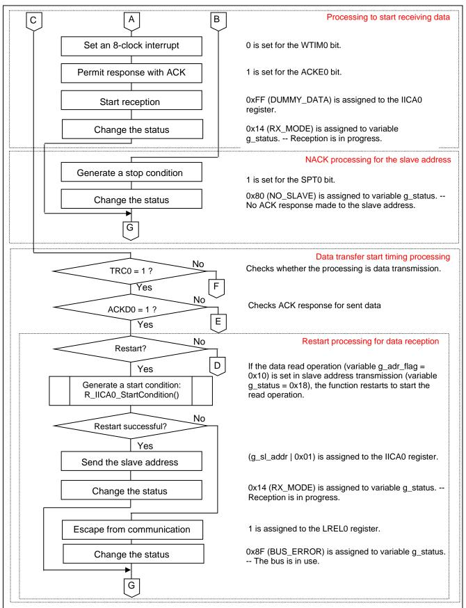
Figure 4-8 IICA0 Master Interrupt Processing Function (3/4)
