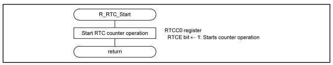
Figure 4.7 RTC Start Setting
