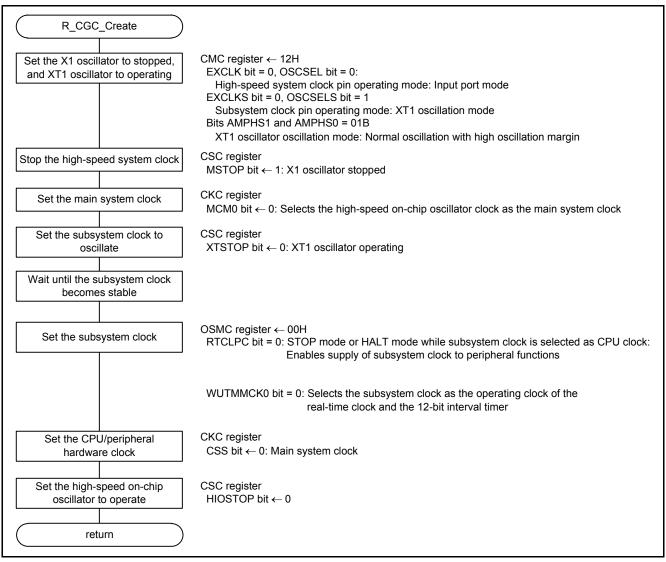
Figure 4.5 CPU Clock Initialization
