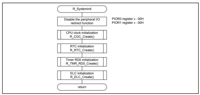
Figure 4.4 Peripheral Function Initialization
