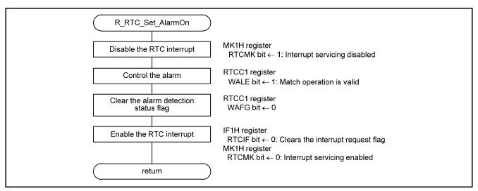
Figure 4.8 Enabling the RTC Alarm Function
