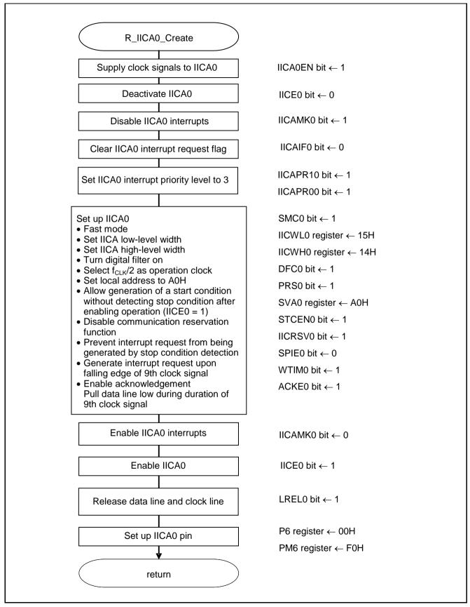
Figure 5.6 Serial Interface IICA Setup
