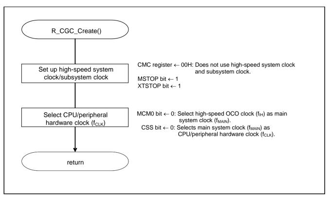
Figure 5.5 CPU Clock Setup
