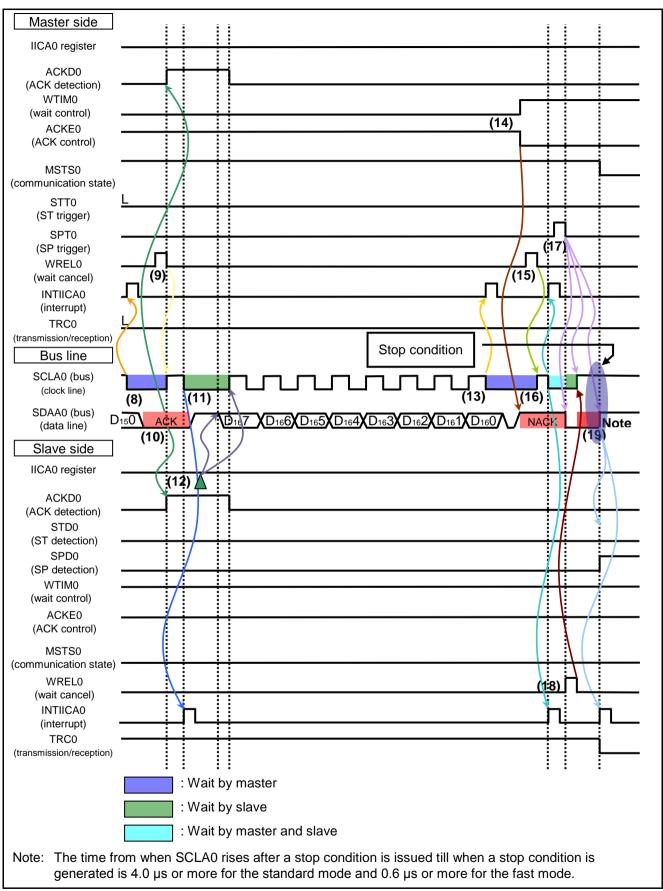
IIC Communication Timing Chart (Slave-to-Master Communication Example) (3/3)
