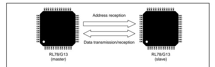
Address reception: Each device connected to the IIC bus has a unique address. Each device receives the address of a transfer destination (slave) from the master. That is, it receives one byte of data consisting of 7 bits (indicating the address) and 1 bit (indicating the transfer direction). The slave generates an acknowledgement after receiving one byte of data.
