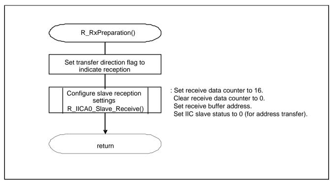
Figure 5.8 IICA0 Reception Preparation Function
