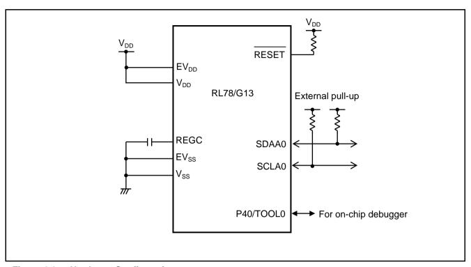
Figure 4.1 Hardware Configuration
