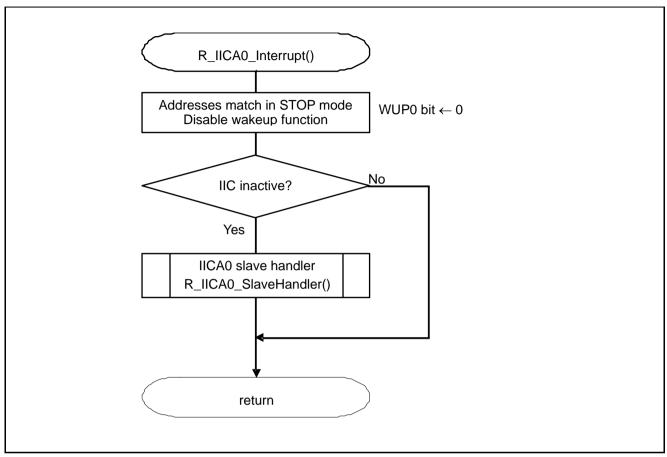
Figure 5.10 IICA0 Interrupt Processing
