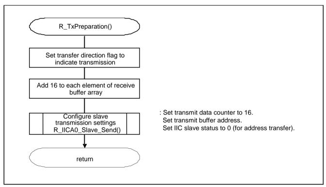
Figure 5.9 IICA0 Transmission Preparation Function
