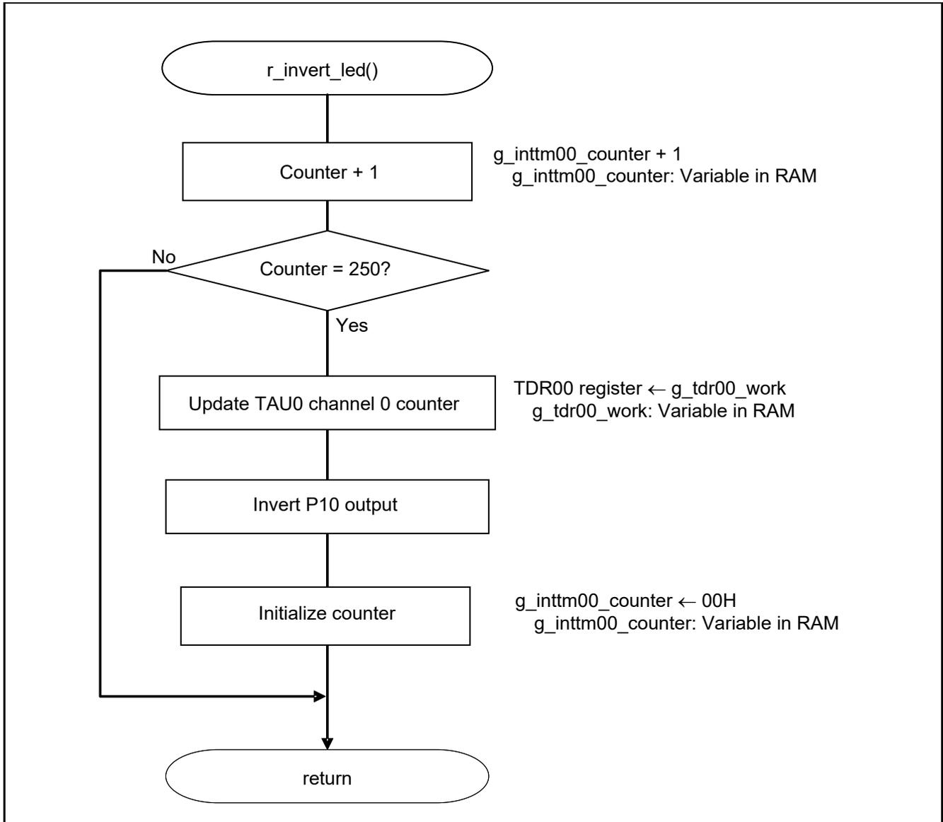
Figure 5.113 Checking Whether 500 ms Have Elapsed
