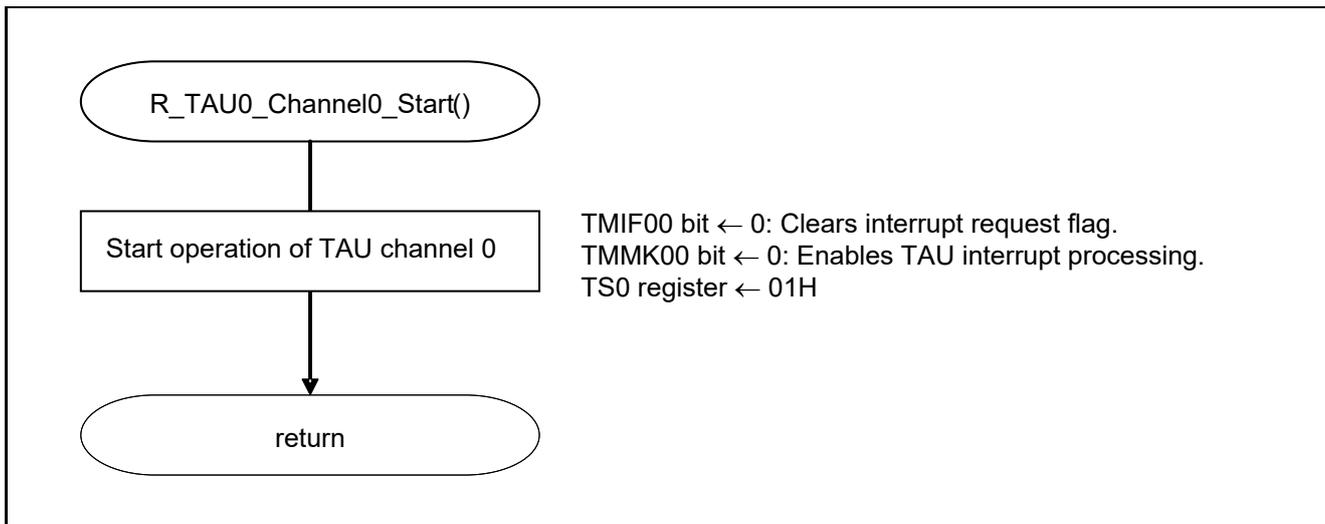
Figure 5.9 Timer Array Unit 0 Operation Start
