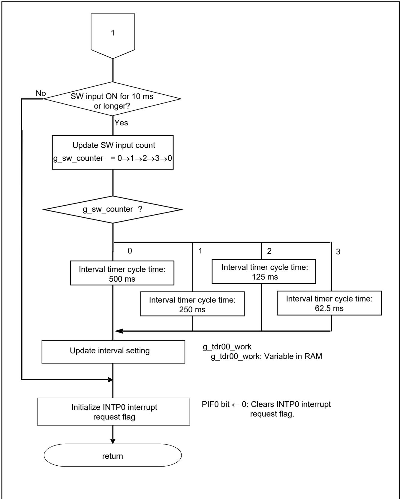
Figure 5.13 INTP0 Interrupt Processing (2/2)
