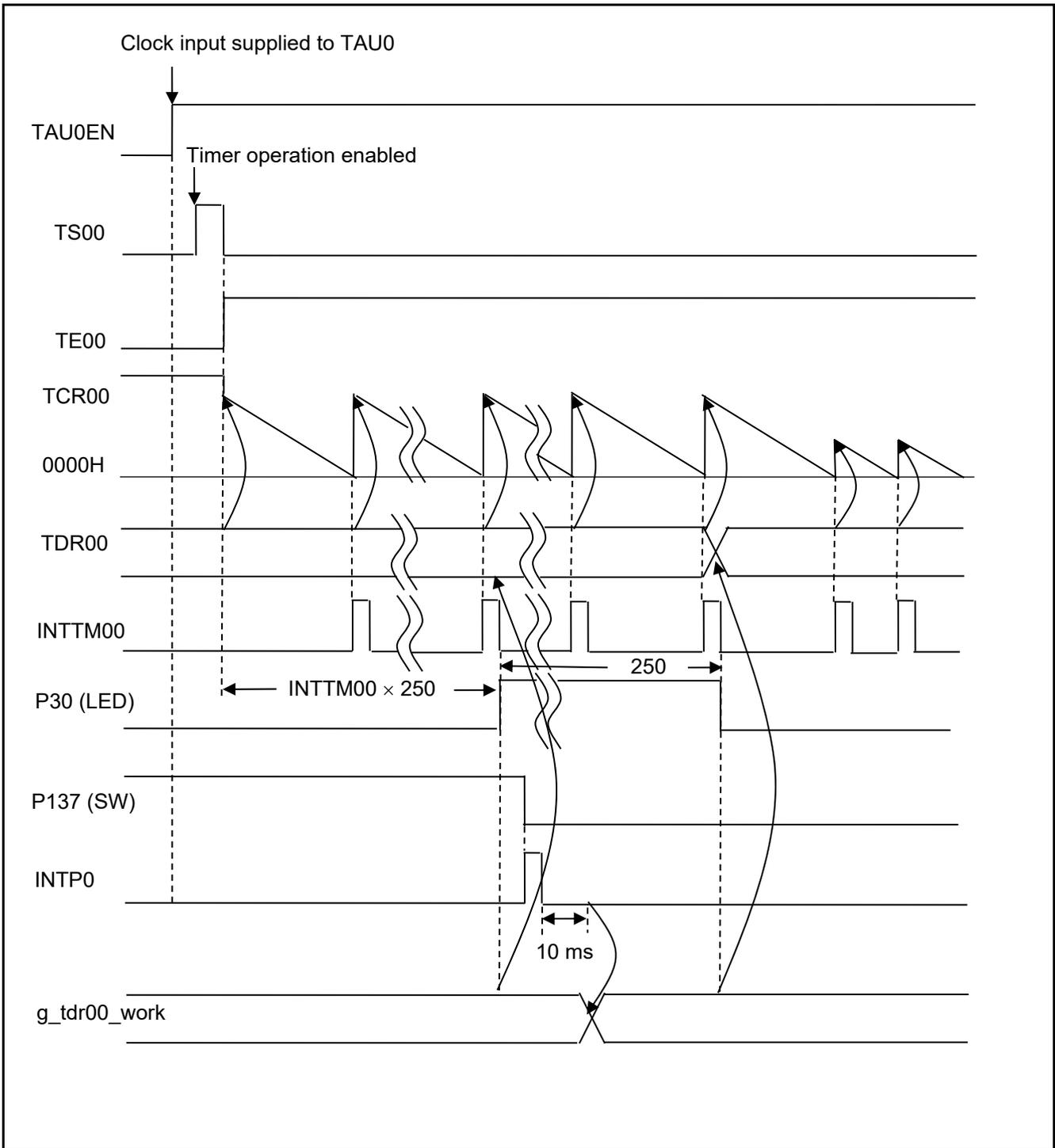
Figure 1.1 Overview of Timer Operation and Interrupts
