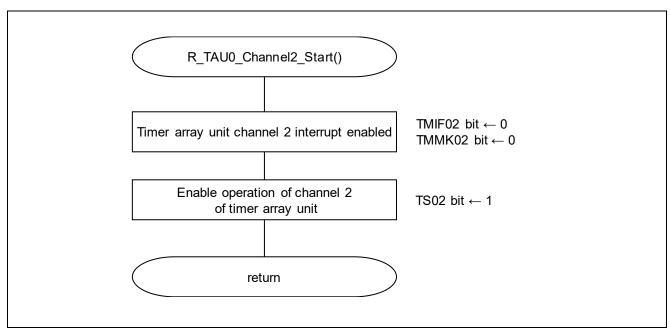
Figure 5.24 Timer Array Unit Channel2 Operation Start Function
