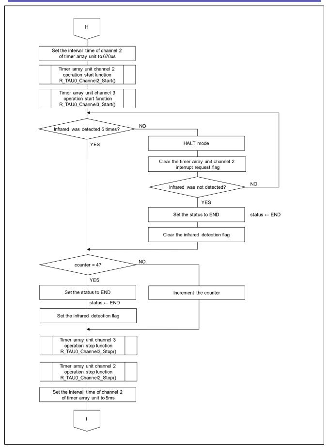
Figure 5.17 Infrared Detection Processing (2/2)
