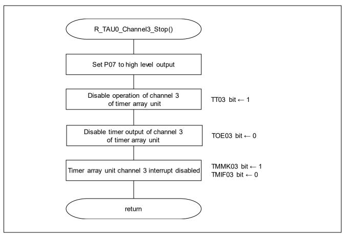
Figure 5.27 Timer Array Unit Channel3 Operation Stop Function
