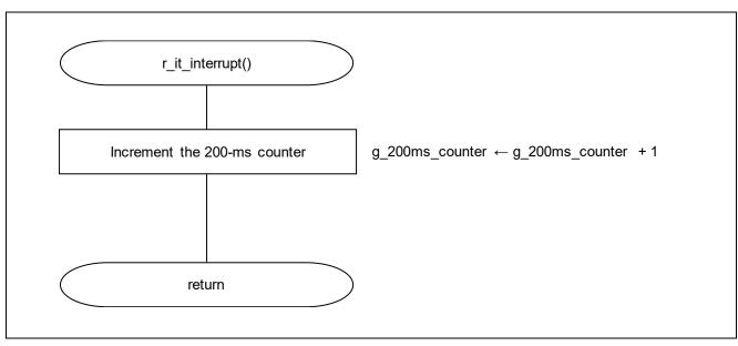
Figure 5.28 Interval Timer Signal Detection Interrupt Function
