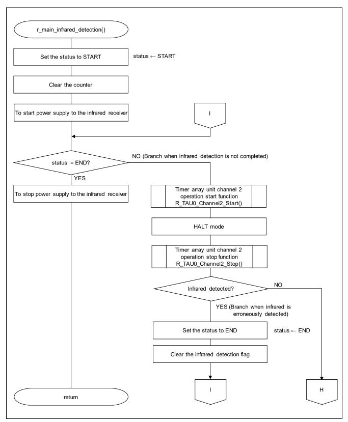
Figure 5.16 Infrared Detection Processing (1/2)
