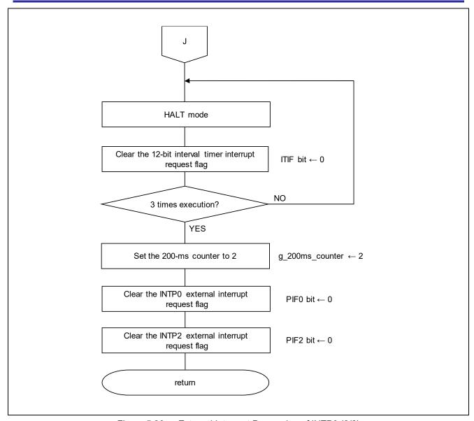
Figure 5.30 External Interrupt Processing of INTP0 (2/2)
