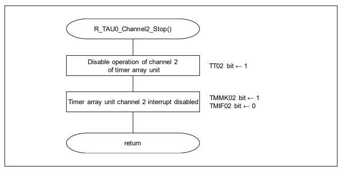
Figure 5.25 Timer Array Unit Channel2 Operation Stop Function
