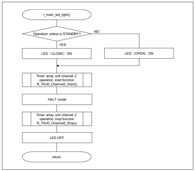
Figure 5.18 LED Blinking Processing
