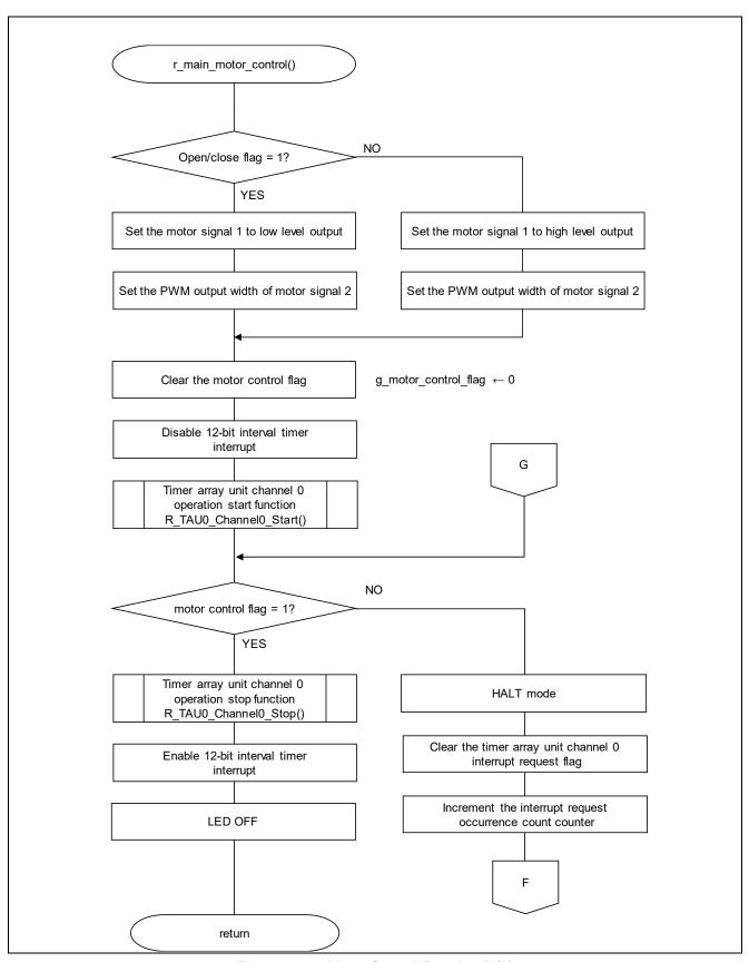
Figure 5.14 Motor Control Function (1/2)
