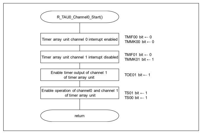
Figure 5.22 Timer Array Unit Channel0 Operation Start Function
