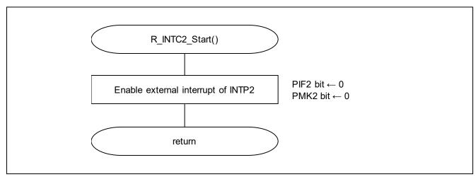
Figure 5.20 External Interrupt Processing of INTP2
