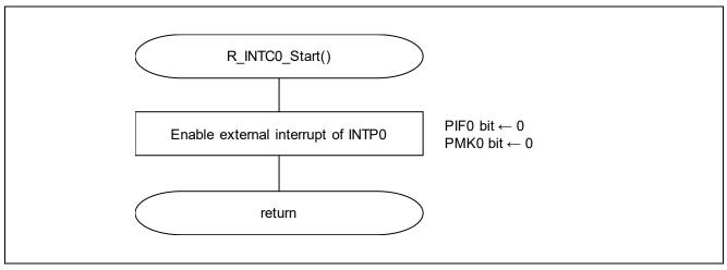
Figure 5.19 External Interrupt Processing of INTP0
