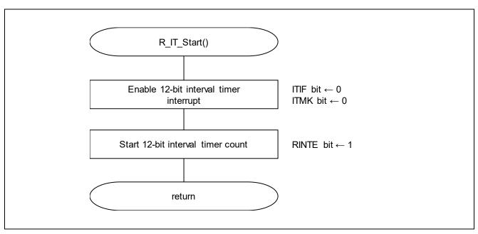
Figure 5.21 12-bit Interval Timer Operation Start
