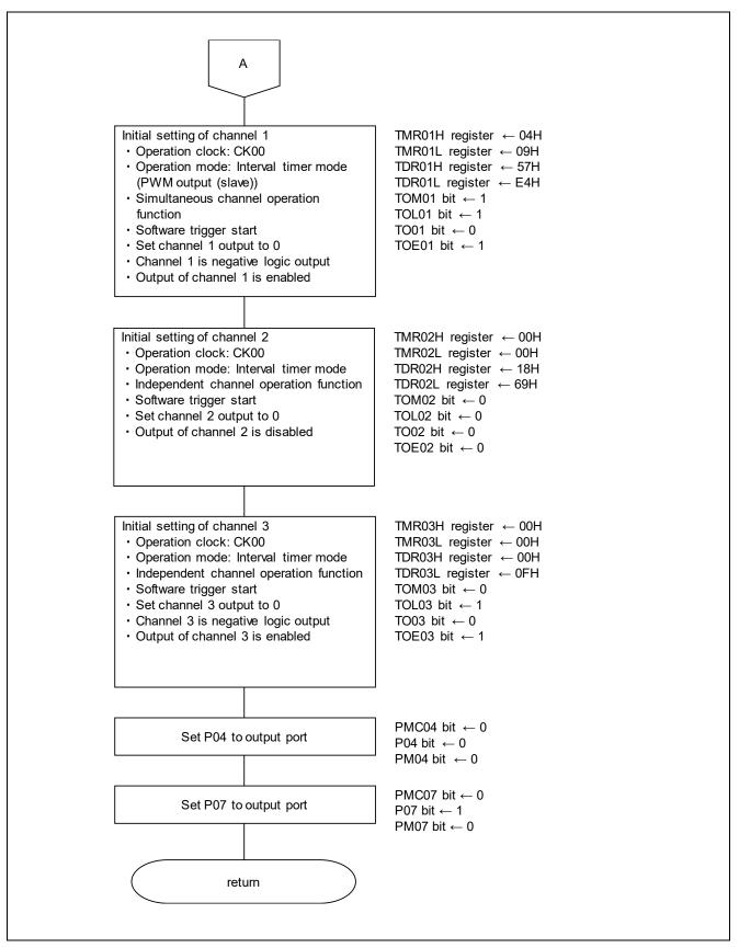
Figure 5.7 Timer Array Unit Initial Setting (2/2)
