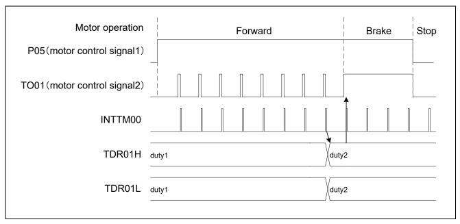
Figure 1.3 Motor Control to Close the Lid
