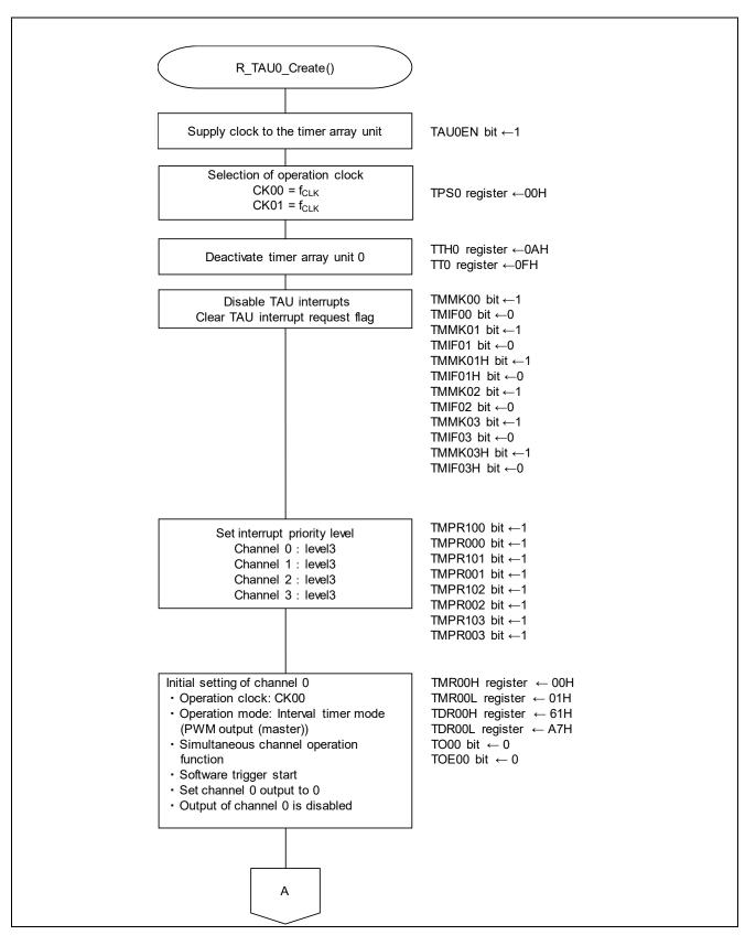
Figure 5.6 Timer Array Unit Initial Setting (1/2)
