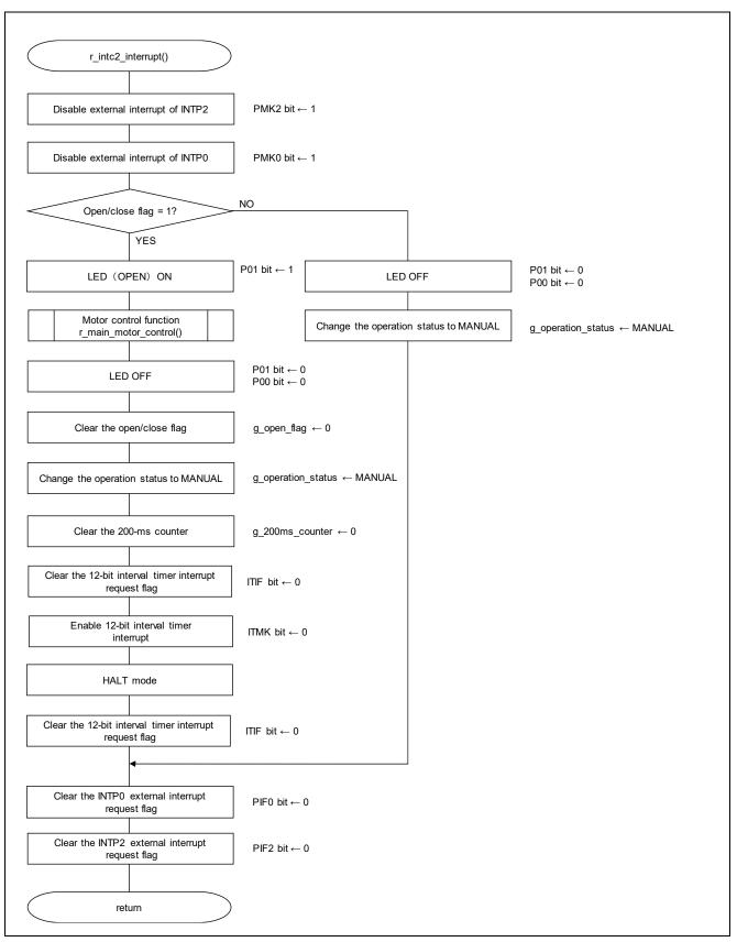
Figure 5.31 External Interrupt Processing of INTP2
