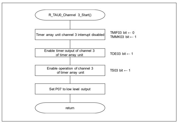
Figure 5.26 Timer Array Unit Channel3 Operation Start Function
