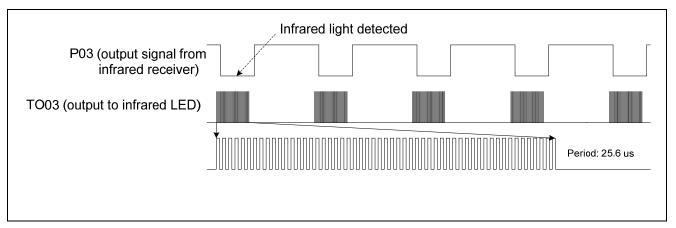
Figure 1.2 Infrared Detection
