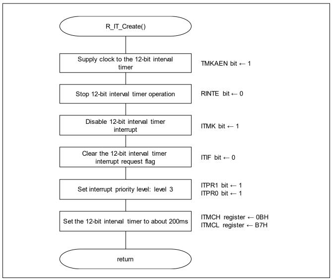
Figure 5.9 12-bit Interval Timer Initial Setting
