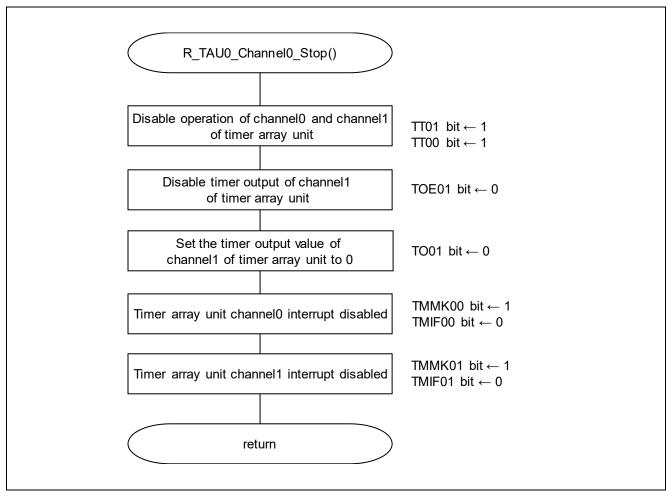
Figure 5.23 Timer Array Unit Channel Operation Stop Function
