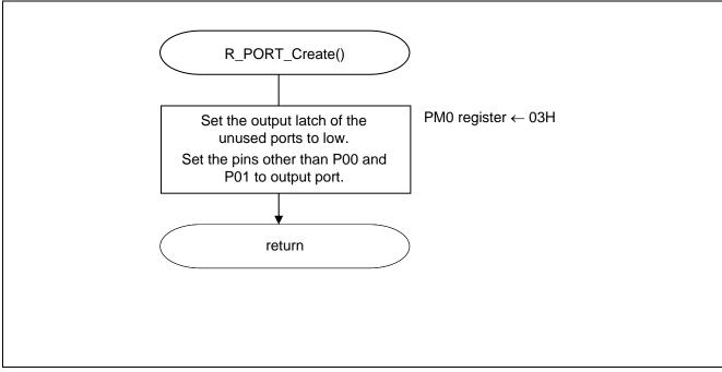
Figure 5.4 I/O Port Setup
