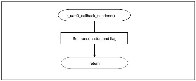
Figure 5.22 UART0 Transmission End Processing Function
