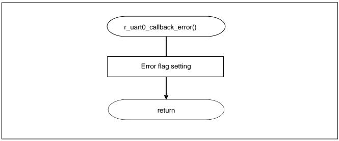
Figure 5.20 UART0 Reception Error Classification Function
