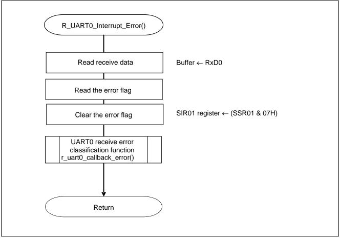
Figure 5.19 UART0 Reception Error Interrupt Function
