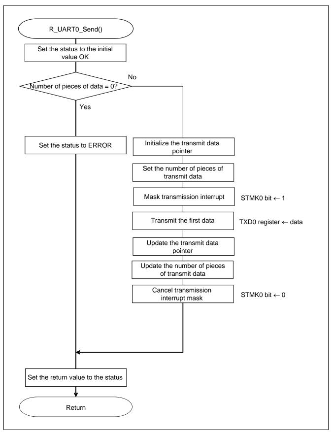
Figure 5.18 UART0 Data Transmission Function
