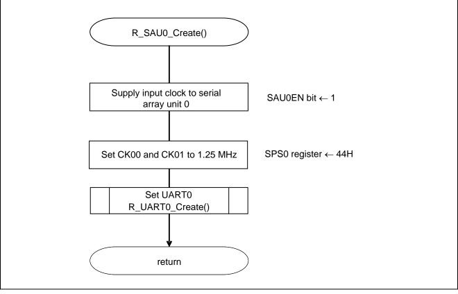
Figure 5.6 Serial Array Unit Setup
