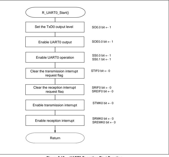
Figure 5.15 UART0 Operation Start Function
