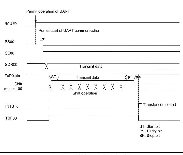
Figure 1.2 UART Transmission Timing Chart
