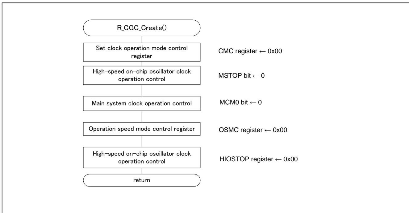
Figure 5.4 CPU Clock Setup
