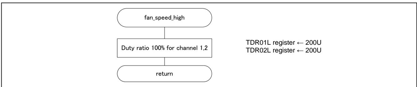
**Figure 5.12 Flowchart of fan high speed**
