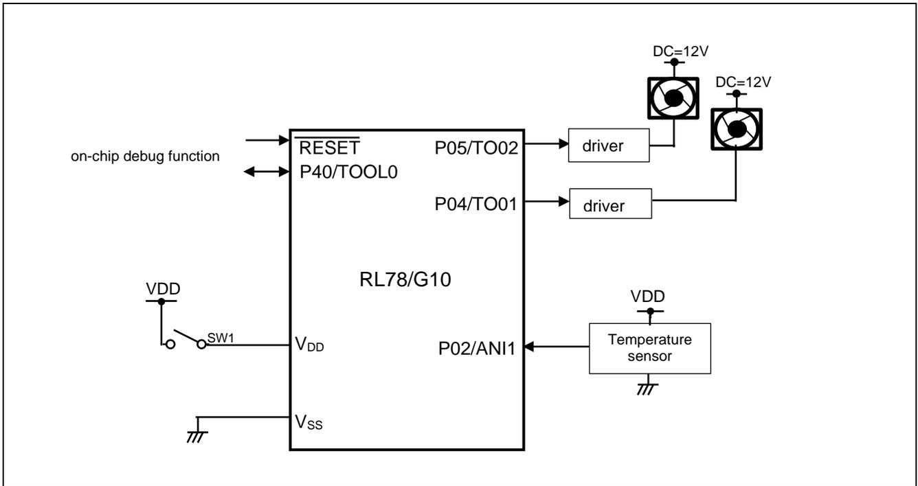
**Figure 4.1 the hardware configuration used for this application**
