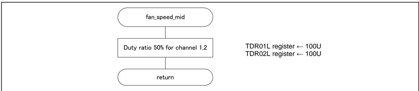
**Figure 5.11 Flowchart of fan middle speed**
