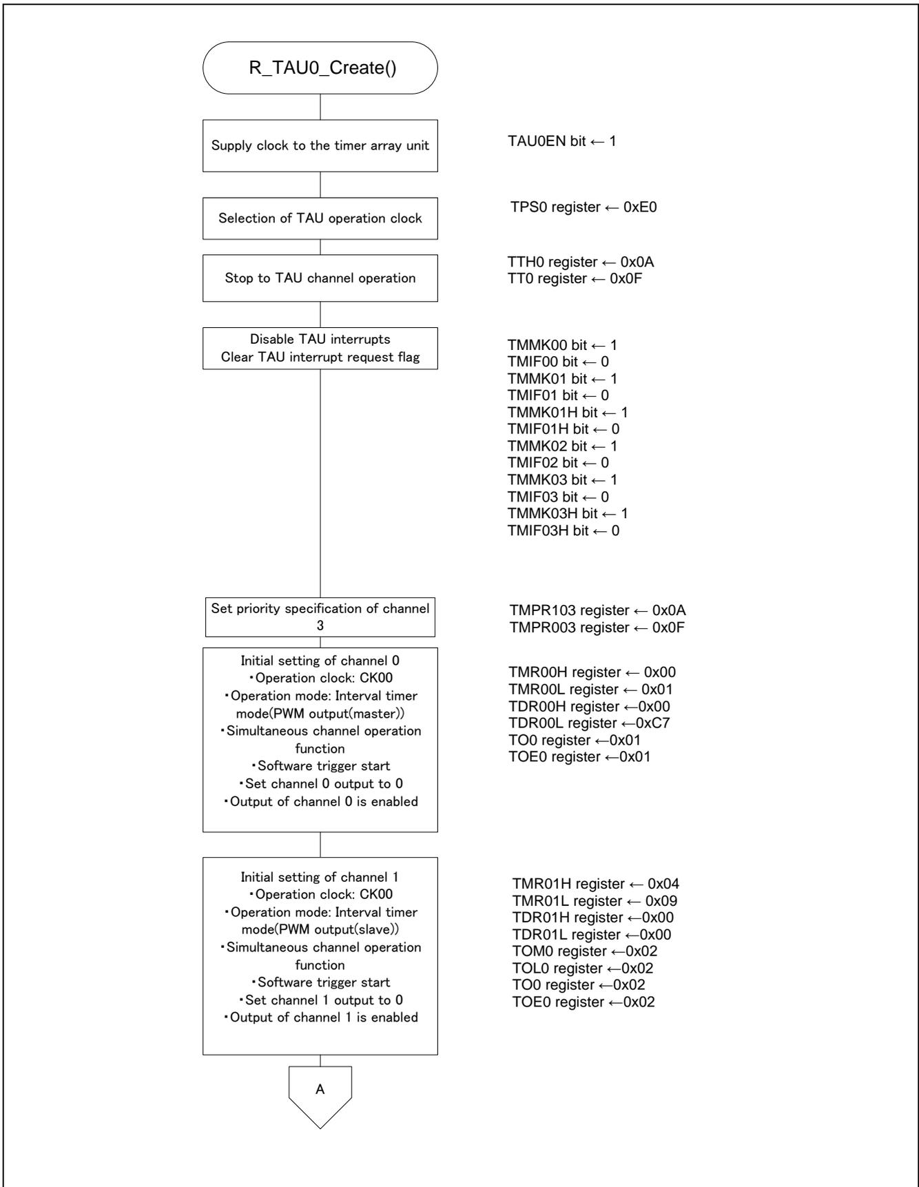
Figure 5.6 Timer Array Unit Setup (1/2)
