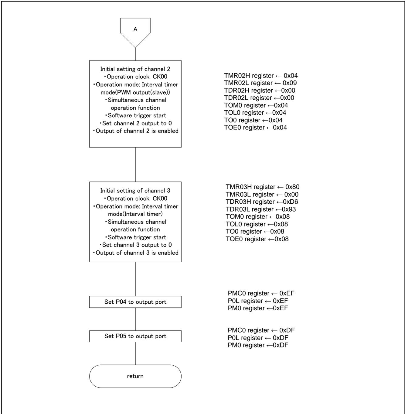
Figure 5.7 Timer Array Unit Setup (2/2)
