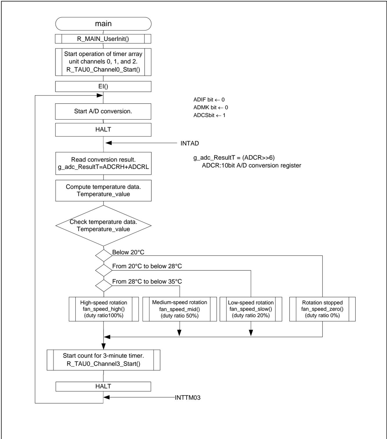
Figure 5.8 Main Processing Flowchart
