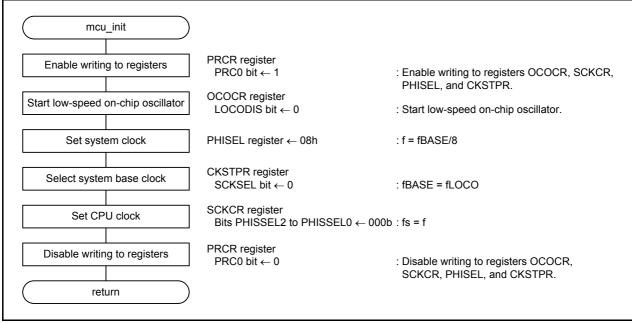
Figure 4.3 System Clock Setting
