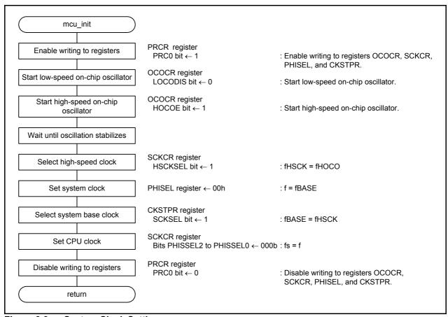
Figure 3.3 System Clock Setting
