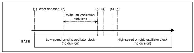
Figure 3.1 Timing Diagram of the Sample Program 1 Setting
