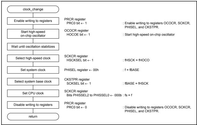
Figure 6.4 System Base Clock Switching
