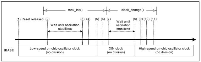
Figure 6.1 Timing Diagram of the Sample Program 4 Setting
