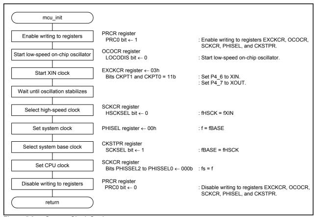
Figure 5.3 System Clock Setting
