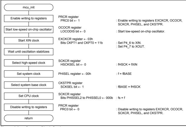
Figure 6.3 System Clock Setting
