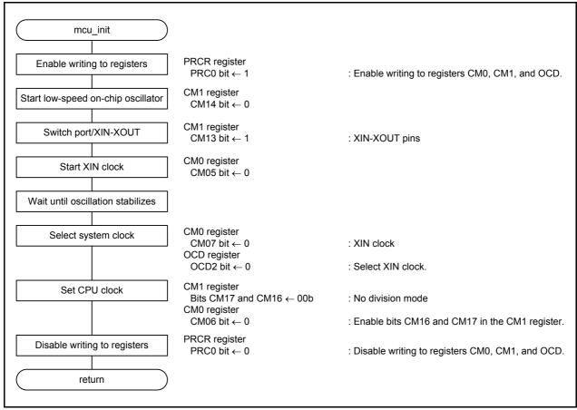
Figure 3.3 System Clock Setting
