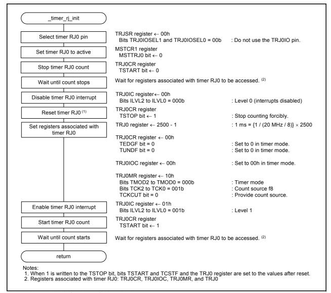
Figure 3.4 Initial Setting of Timer RJ0
