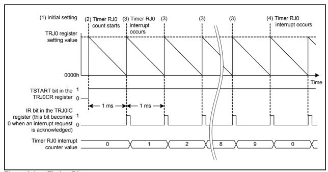
Figure 3.1 Timing Diagram
