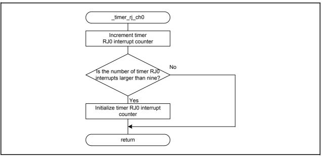
Figure 3.5 Timer RJ0 Interrupt Handling
