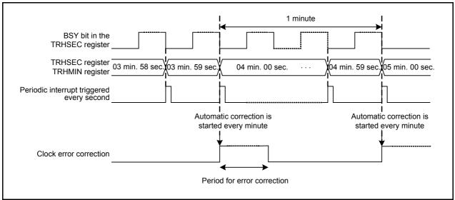
Figure 1.2 Operating Example of Automatic Correction Function and Correction to the Minus Side
