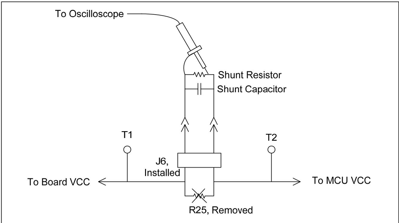
**Figure 2. Configuration of current measurement with oscilloscope**
