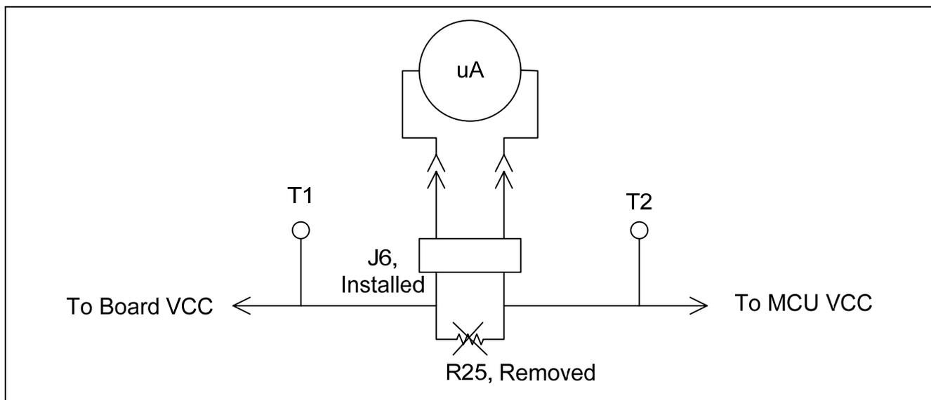
Figure 1. Simplified schematic of MCU current test points
