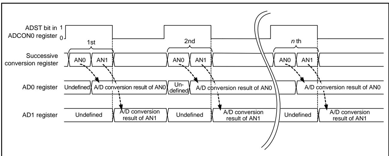
Figure 3.2 Operation in Single Sweep Mode
