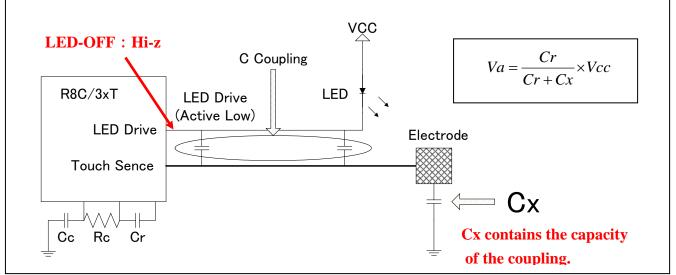
Figure 1-1 Influence when electrode signal line runs side by side with other signal wires
