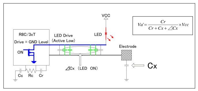
Figure 1-3 Influence when electrode signal line runs side by side with other signal wires (LED is ON)
