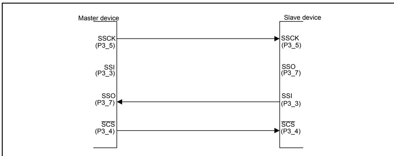
Figure 3.2 Connections in 4-Wire Bus Communication (Bidirectional) Mode
