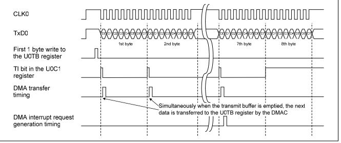
Figure 2. Successive Transmission/reception Timing
