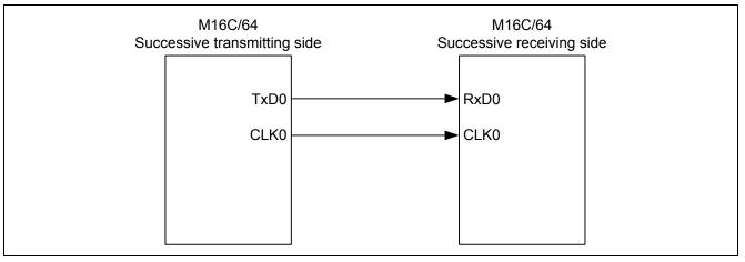
Figure 1. Example Connection for Successive Transmission/Reception
