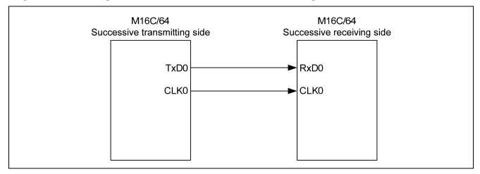
Figure 1. Example Connection for Successive Transmission/Reception
