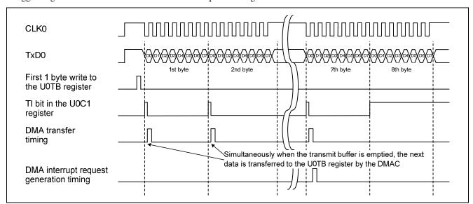
Figure 2. Successive Transmission/reception Timing
