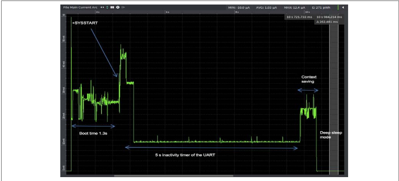
Figure 10. Power Graph in CFUN=0 Mode
