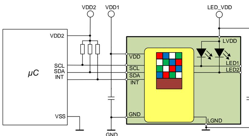
Figure 1. Application Circuit
