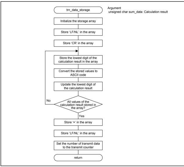
Figure 4.6 Processing for Transmit Data Storage
