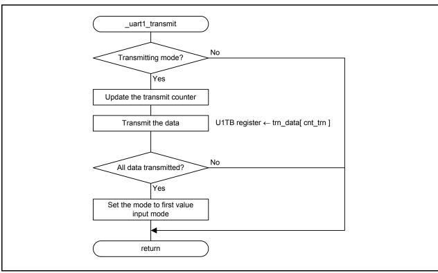
Figure 4.7 UART1 Transmit Interrupt Handler
