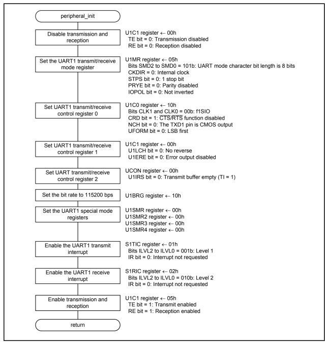
Figure 4.3 Peripheral Function Initialization
