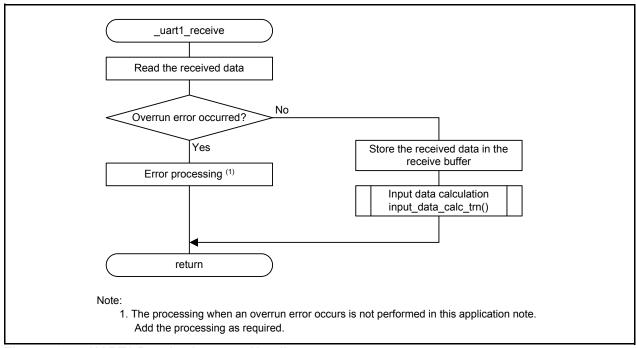
Figure 4.8 UART1 Receive Interrupt Handler
