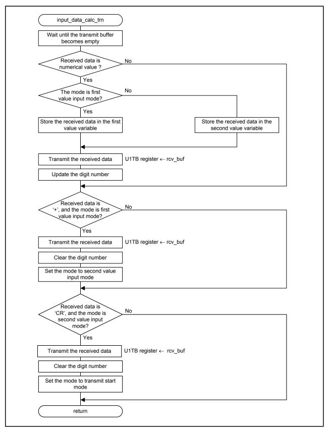
Figure 4.9 Input Data Calculation Transmission
