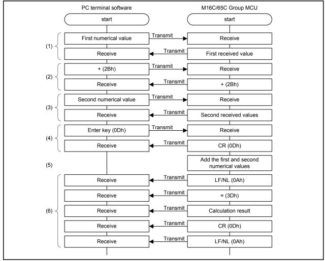
Figure 4.1 Overview of the PC Terminal Software and Sample Code Operations
