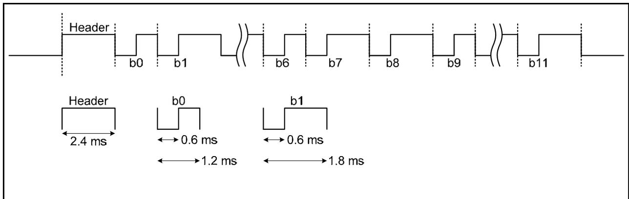
Figure 1.2 Pattern B: Remote Control Format with Special Header Pattern
