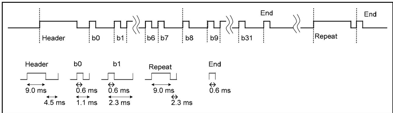
Figure 1.1 Pattern A: Remote Control Format with Header Pattern and Repeat Code
