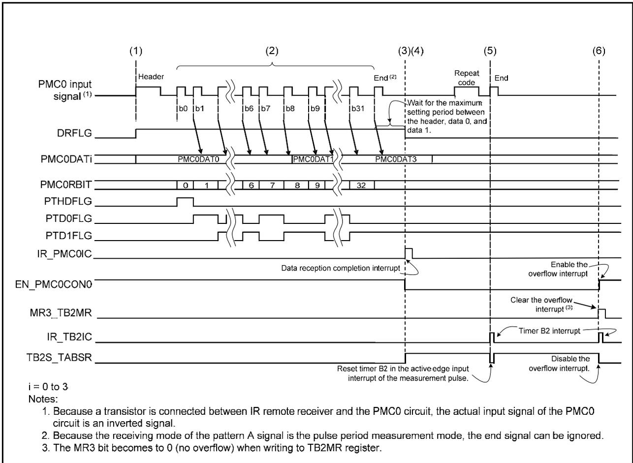
Figure 5.1 PMC0 Reception Timing of the Remote Control with Header and Repeat Code Format
