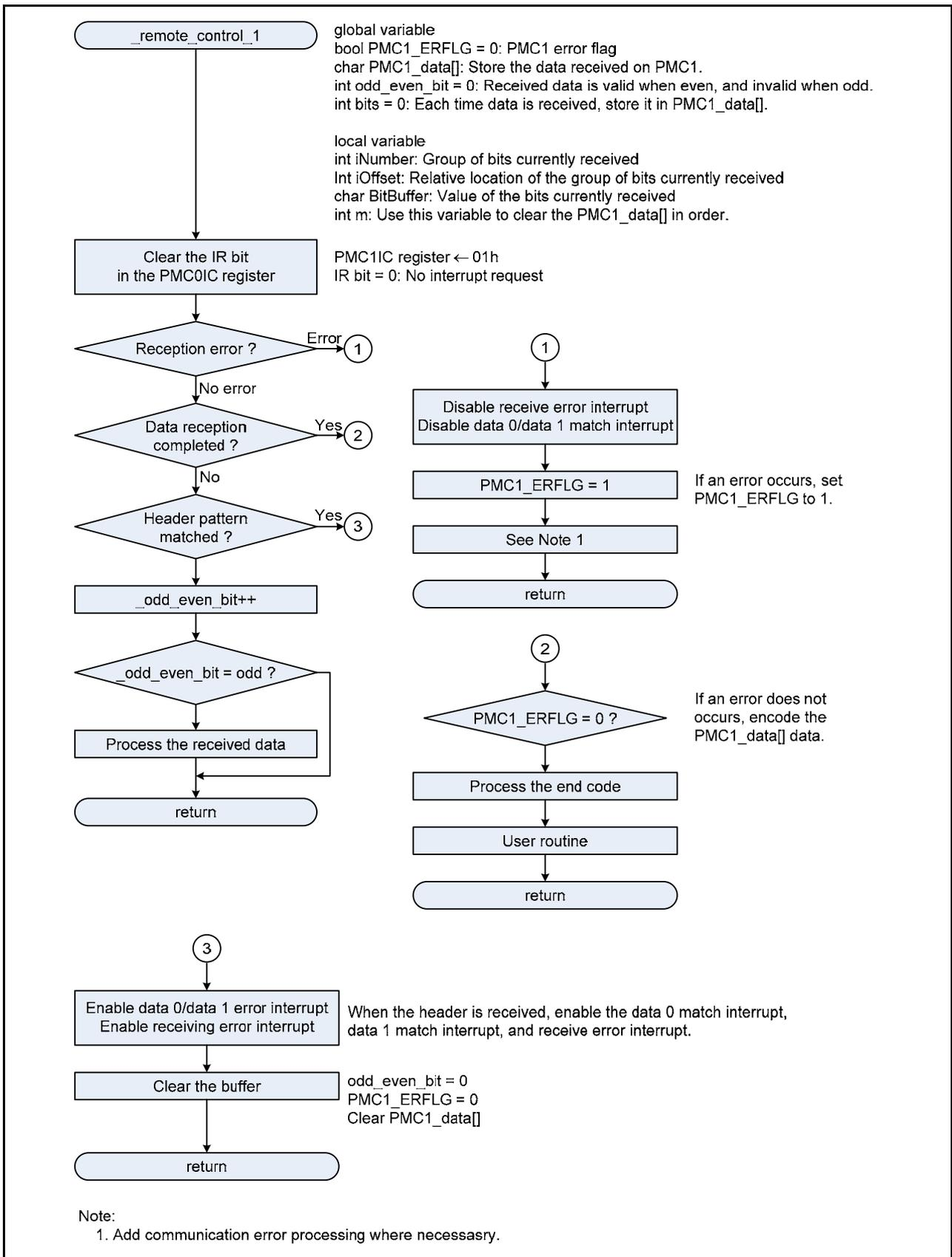
Figure 5.10 PMC1 Interrupt Handling
