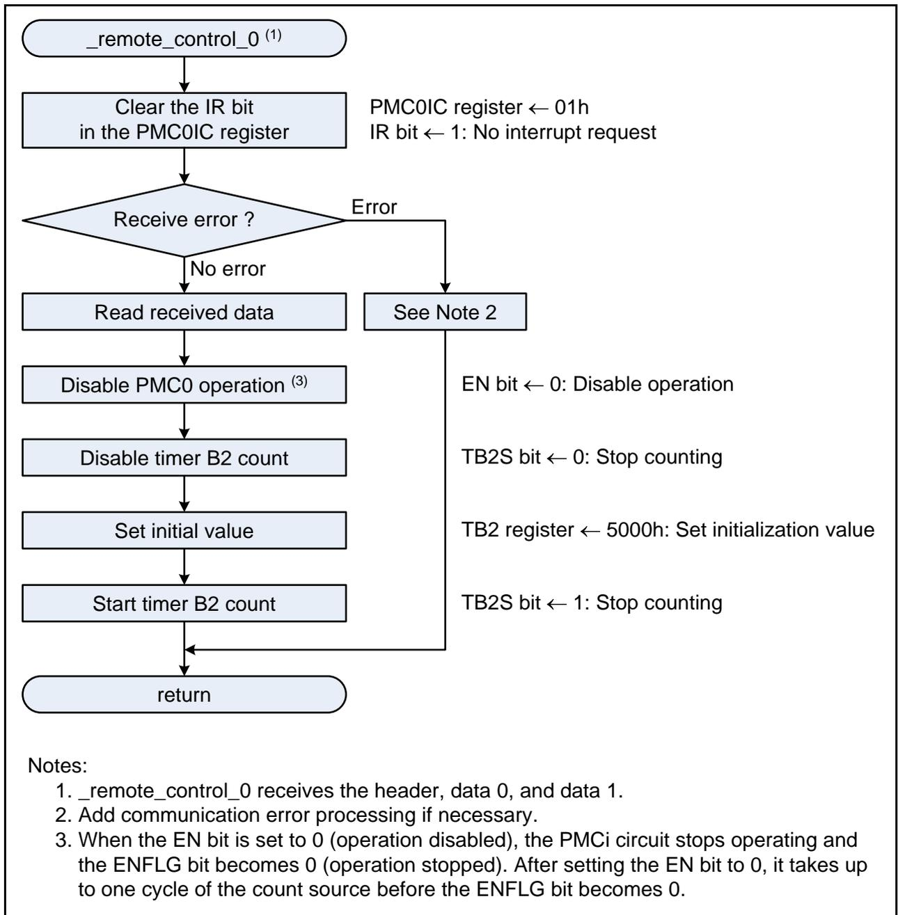
Figure 5.8 PMC0 Interrupt Handling
