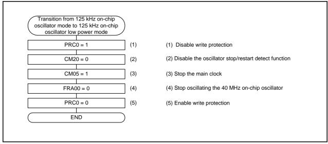
Figure 3.3 Transition from 125 kHz On-Chip Oscillator Mode to 125 kHz On-Chip Oscillator Low Power Mode
