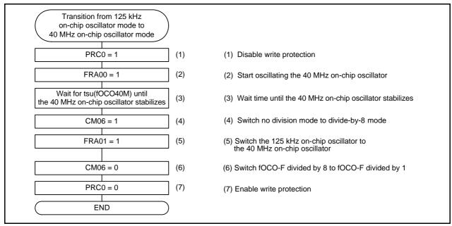
Figure 3.5 Transition from 125 kHz On-Chip Oscillator Mode to 40 MHz On-Chip Oscillator Mode (fOCO-F Divided by 1)
