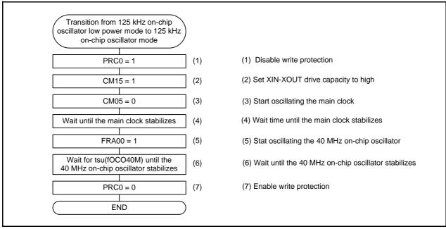
Figure 3.4 Transition from 125 kHz On-Chip Oscillator Low Power Mode to 125 kHz On-Chip Oscillator Mode
