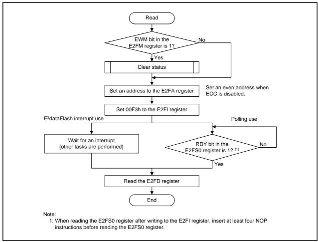
Figure 3.3 Read Operation Example
