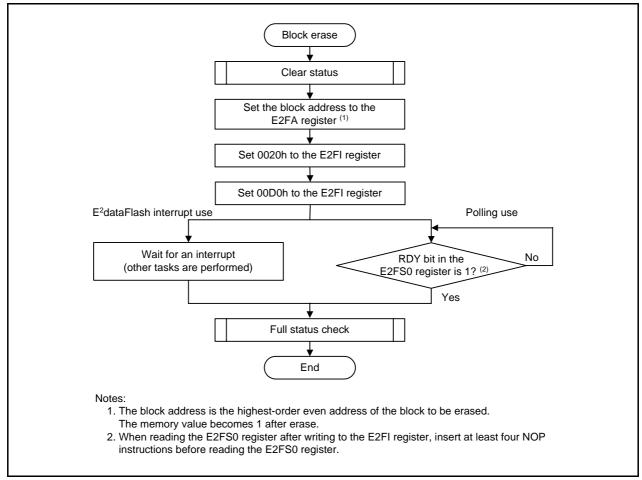
Figure 3.5 **Block Erase Operation Example**
