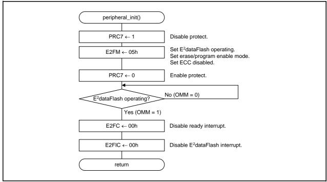
Figure 4.3 Peripheral Function Initial Setting
