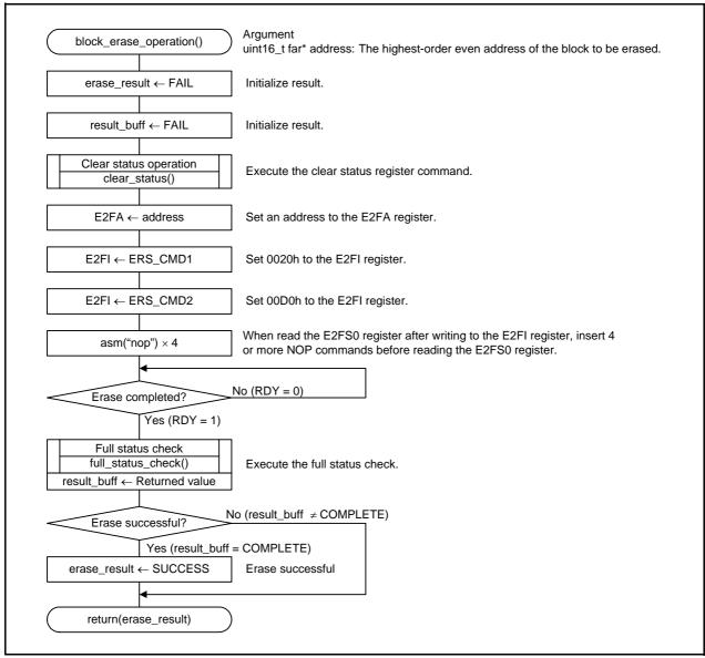
Figure 4.5 Block Erase Operation
